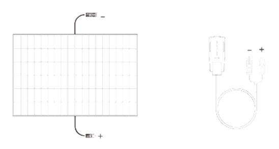
To test the polarities of the wires from the hub: Use the multimeter buzzer to measure the conduction between the P pole of the PV connector and the +, and between the N pole and the - in the figure.
