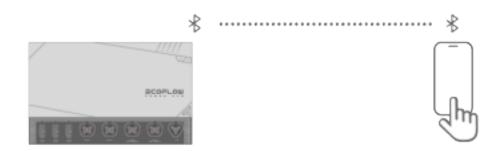
To reset Bluetooth for pairing with the Power Kits using a different phone: Press and hold the DC button on the hub for more than 3 seconds till the ALT input, AC input, and AC output indicators light up in sequence. The 3 indicators will blink for 5 times, indicating the reset is successful.
