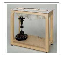
The bottom plate contains three pair of bolts for locking the device holder. The device holder positions are adjusted to the standard measurement positions in the three sections. A white cover is provided to tap the phantom during off-periods to prevent water evaporation and changes in the liquid parameters. On the phantom tip, three reference markers are provided to identify the phantom position with respect to the robot.
