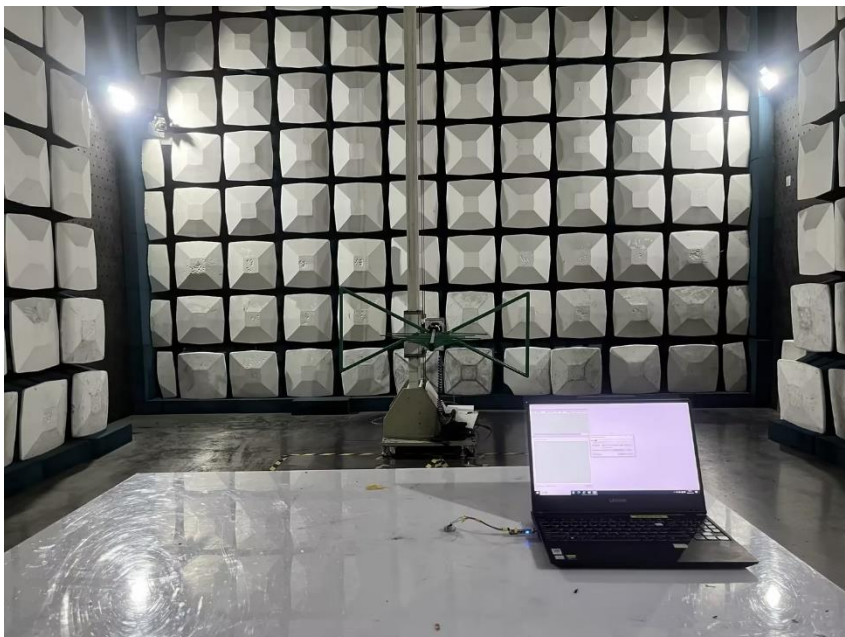
Radiated Test Below 1GHz
