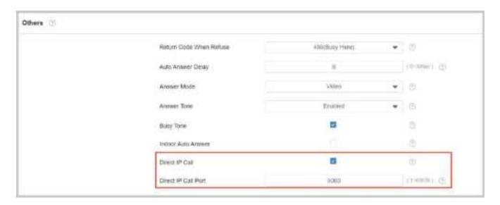
• Direct IP Call Port: The direct IP call port is 5060 by default with the port range from 1-65535. If you enter any values within the range other than 5060, you are required to check if the value entered is consistent with the corresponding value on the device you wish to establish a data transmission.
