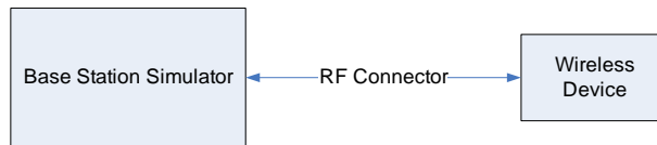
Figure 9-2 Power Measurement Setup
