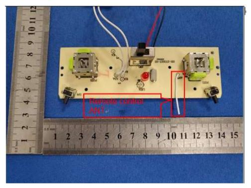
Length: 3.6cm Antenna Type: Wire Antenna Antenna Gain:0dBi
