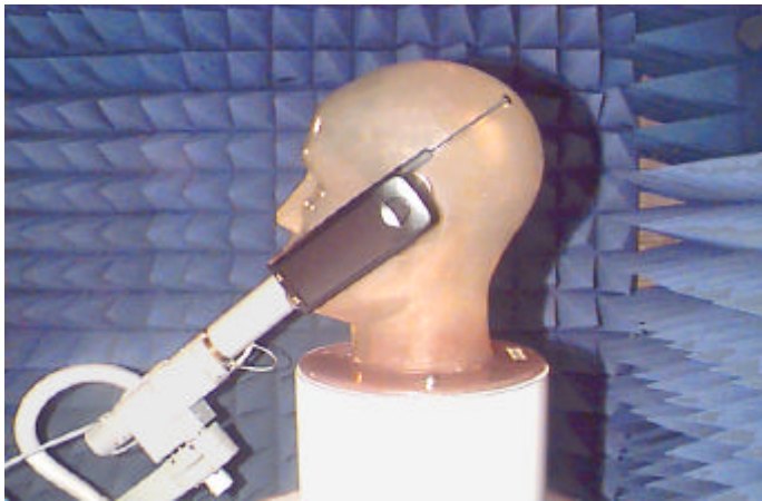
Figure 9. Sample of Handset alignment with the Ear Canal of the Phantom
