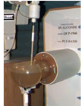
Figure 1. SAR Test Set-up
