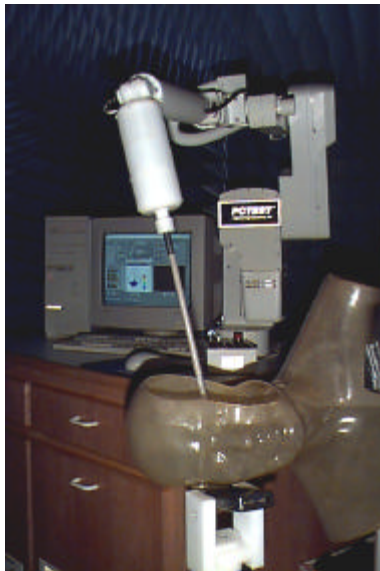
Figure 5. Photograph of the Probe and the Phantom
