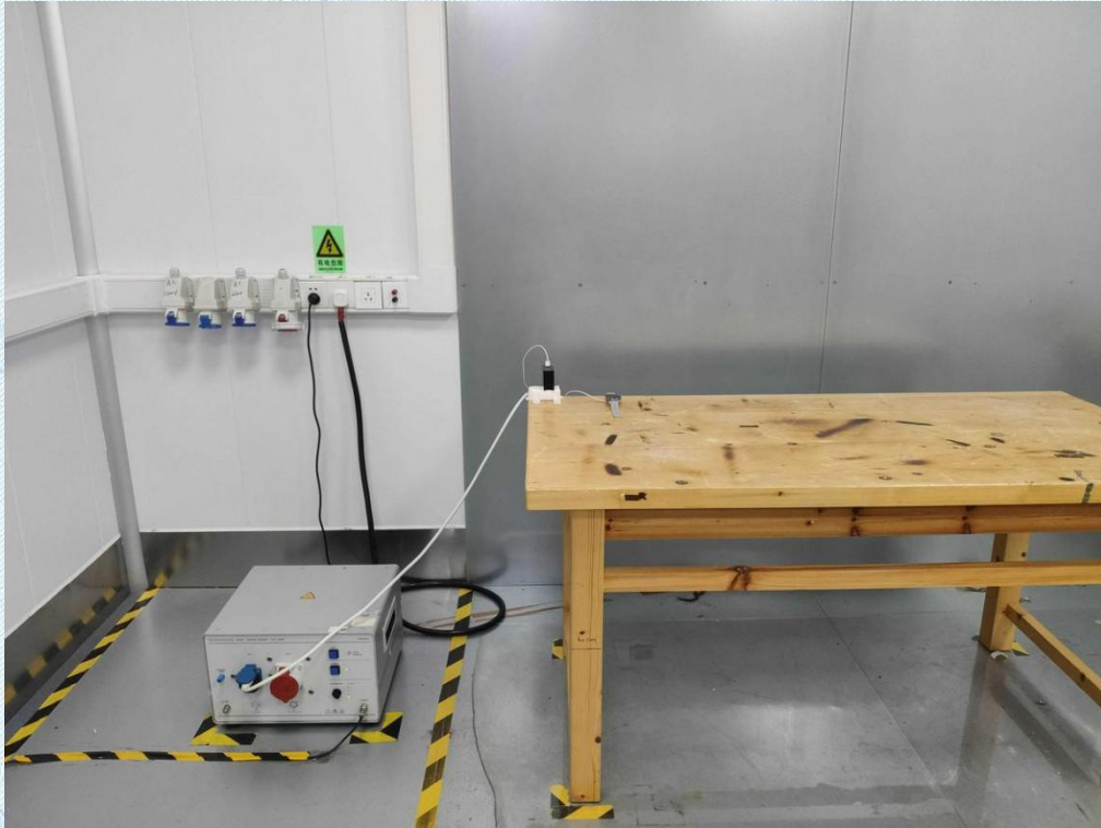
Conducted Emission at AC power line
