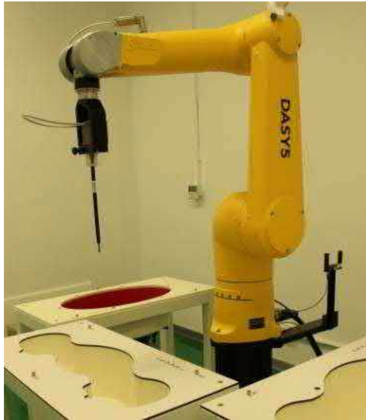
Picture 8.4-1: Specific Absorption Rate Test Layout
