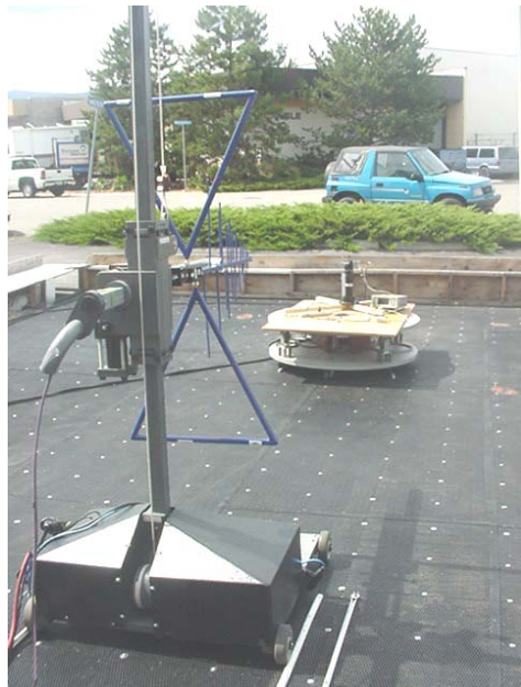
Photograph B.7-7 - Dipole Substitution Setup
