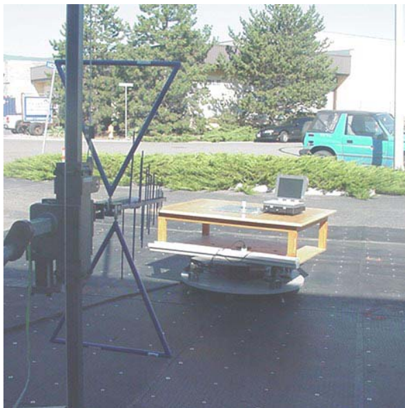
Photograph B.7-7 - Dipole Substitution Setup
