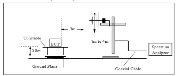
3. Radiated Emission Test-Up Frequency Above 1GHz
