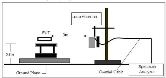
2. Radiated Emission Test-Up Frequency 30MHz~1GHz
