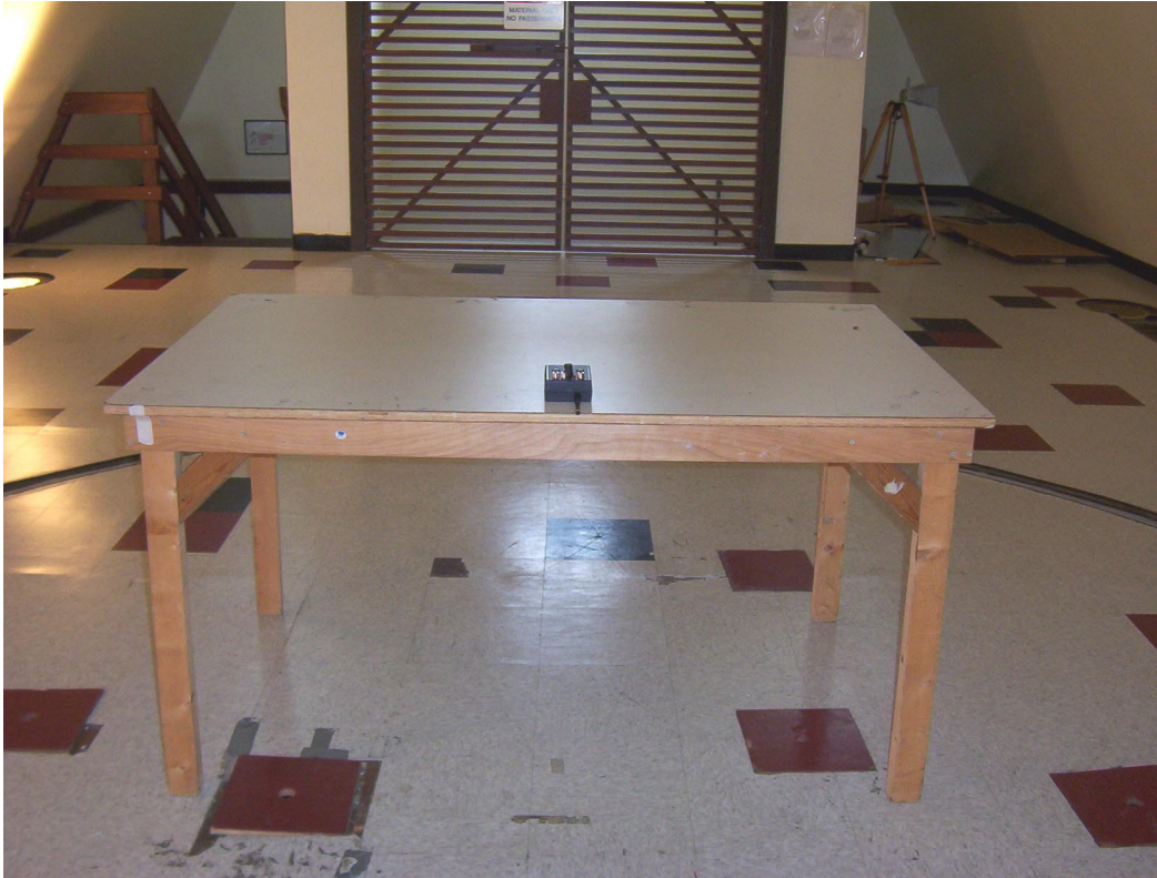
Radiated Emission Test Setup – Flat On Back
