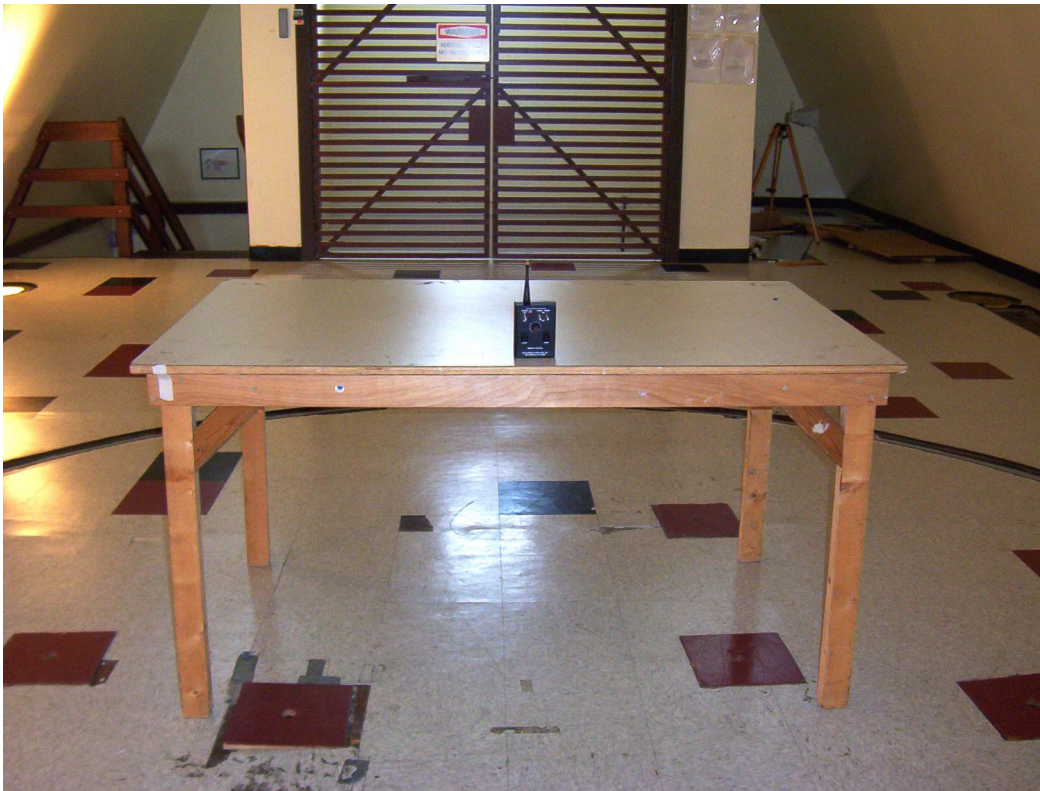
Radiated Emission Test Setup – Front View
