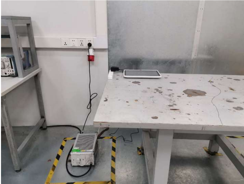
Photo of Power Line Conducted Emission Test
