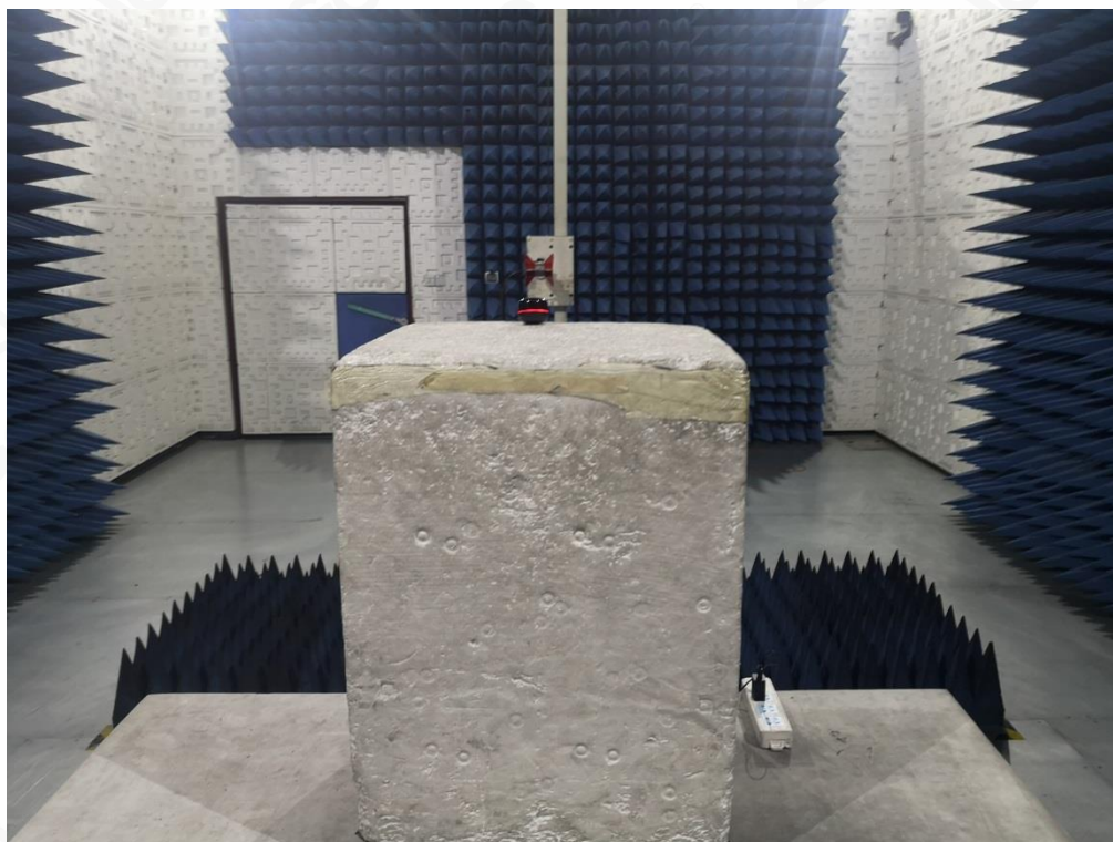
FCC RADIATED EMISSION TEST SETUP ABOVE 1GHZ
