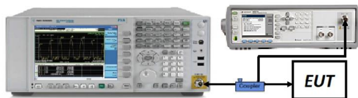
Figure 7-1. Test Instrument & Measurement Setup
