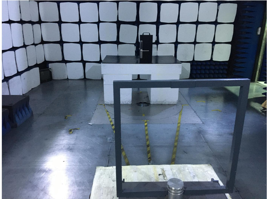
Radiation Emission Test Setup (Below 30MHz)
