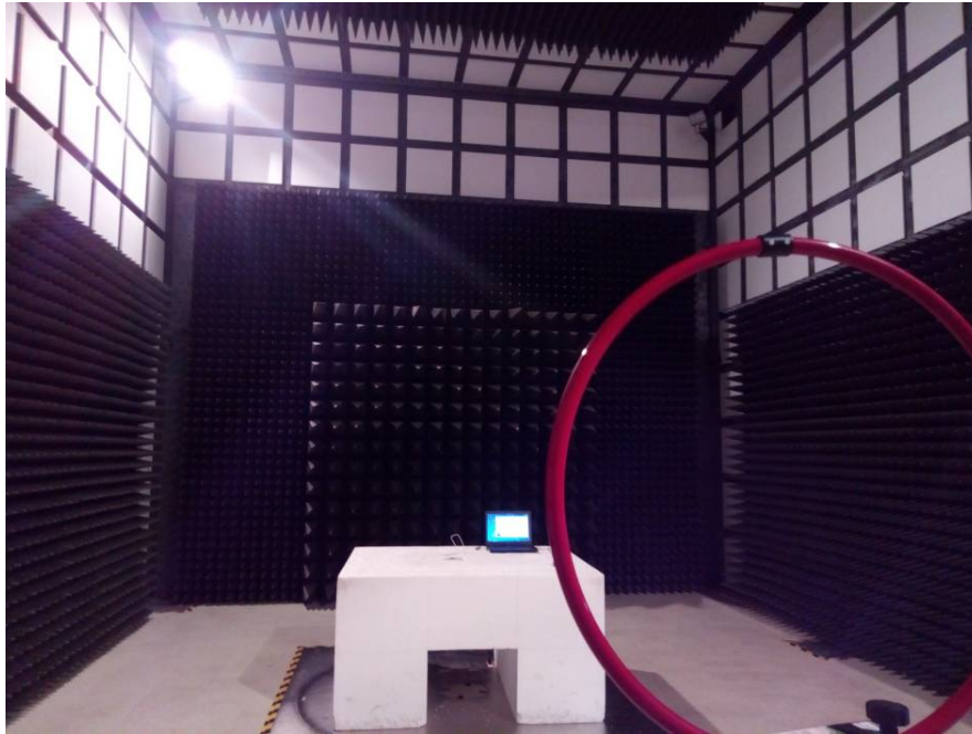
Radiated Emissions View (Below 30 MHz)
