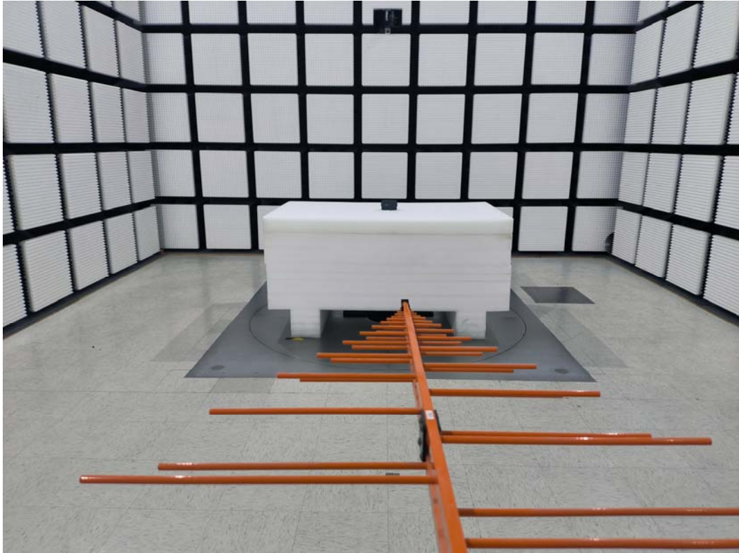
Radiated Emission Above 1GHz View
