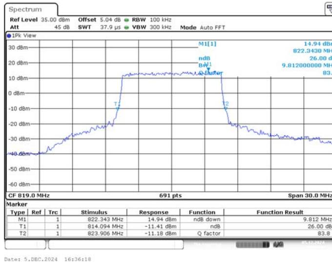
**LTE band 26(824MHz~849MHz),1.4MHz(-26dBc)**
