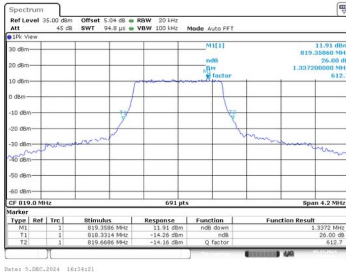
**LTE band 26(814MHz~824MHz),3MHz(-26dBc)**
