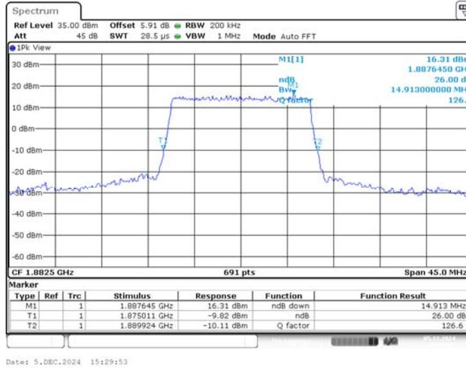
**LTE band 25 , 15MHz Bandwidth,MID,16QAM (-26dBc BW)**
