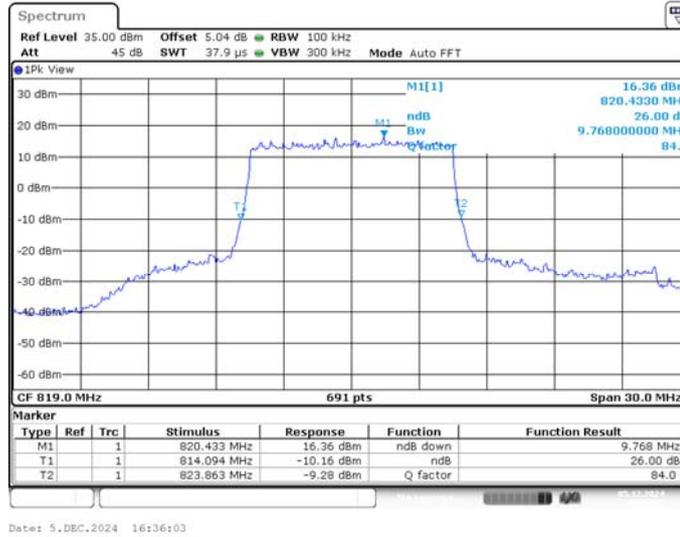
**LTE band 26 , 10MHz Bandwidth,MID,16QAM (-26dBc BW)**
