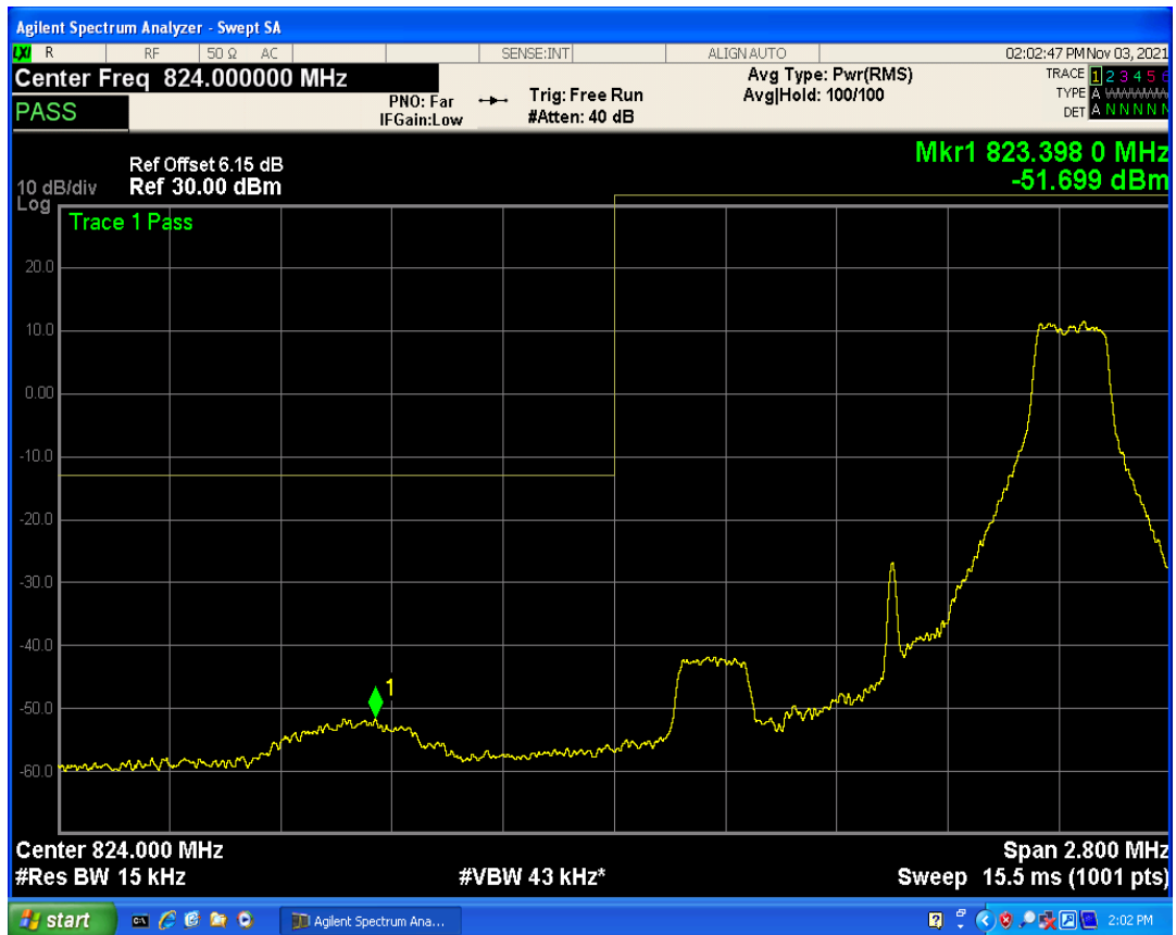
Band5 QPSK BW=1.4MHz Channel=20643 RB Size=1 Position=#0
