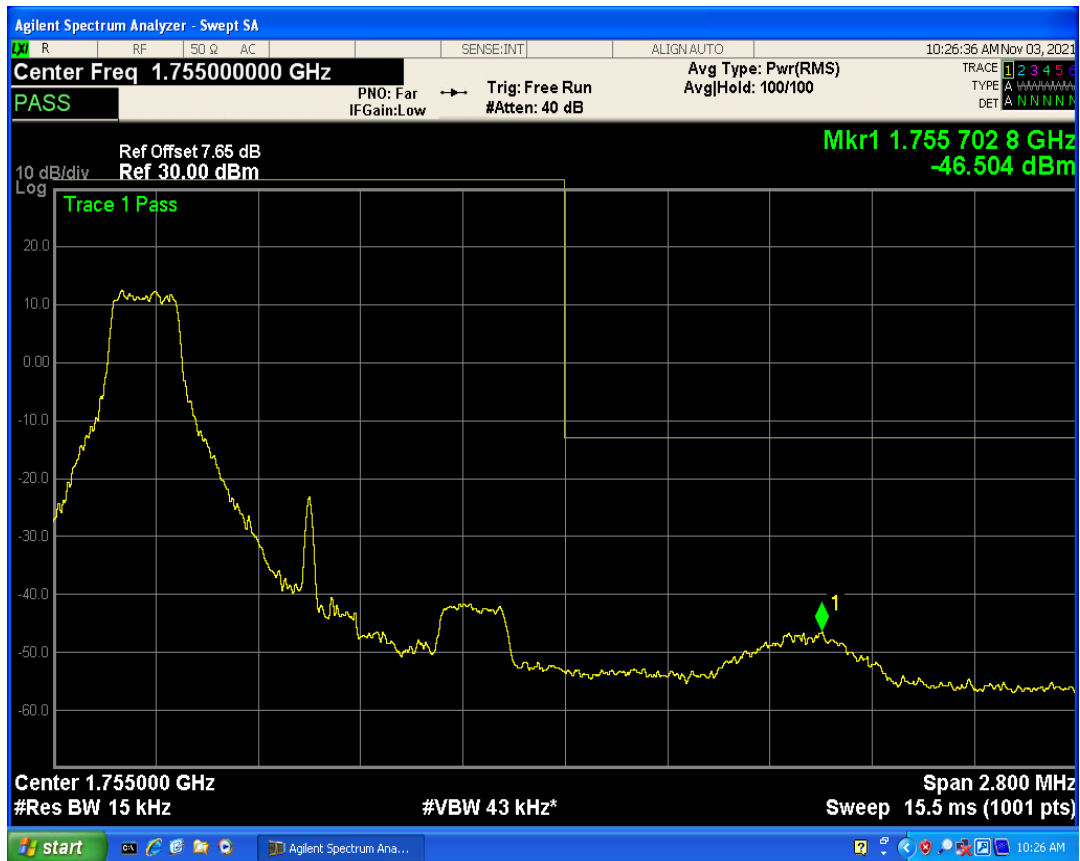
Band4 QPSK BW=1.4MHz Channel=20393 RB Size=6 Position=#0
