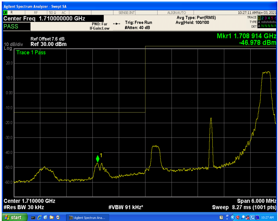
Band4 QAM16 BW=3MHz Channel=19965 RB Size=15 Position=#0
