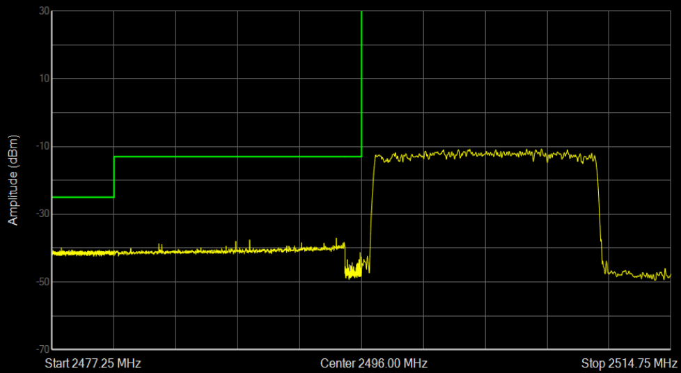
Band41 QAM16 BW=15MHz Channel=39725 RB Size=75 Position=#0
