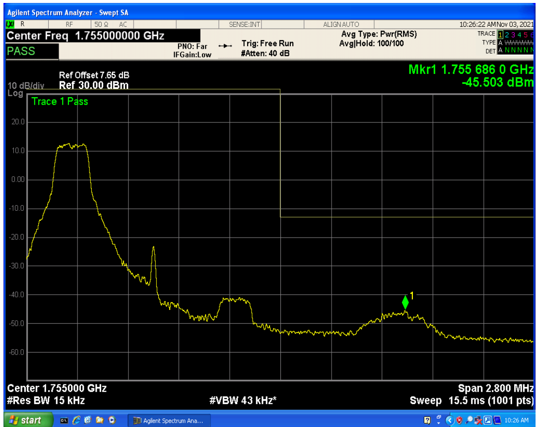
Band4 QPSK BW=1.4MHz Channel=20393 RB Size=1 Position=#Max
