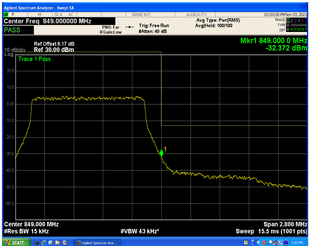
Band5 QAM16 BW=1.4MHz Channel=20643 RB Size=1 Position=#Max
