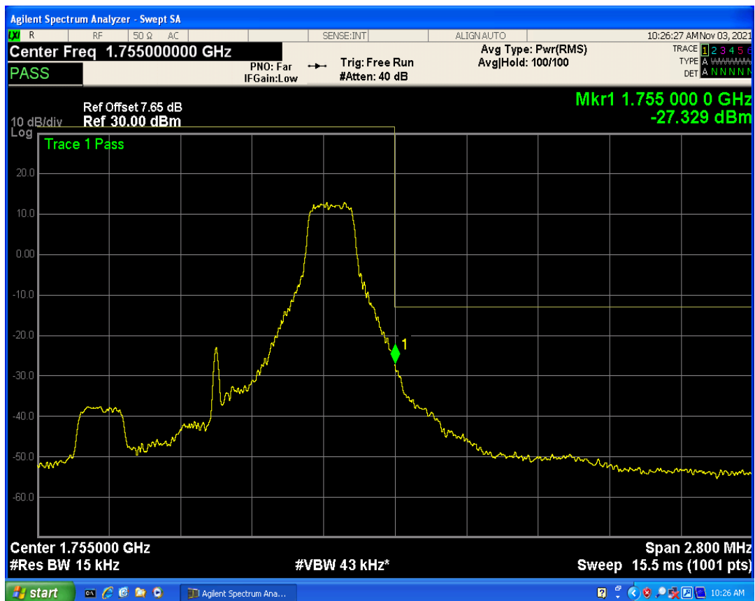
Band4 QAM16 BW=1.4MHz Channel=20393 RB Size=1 Position=#0
