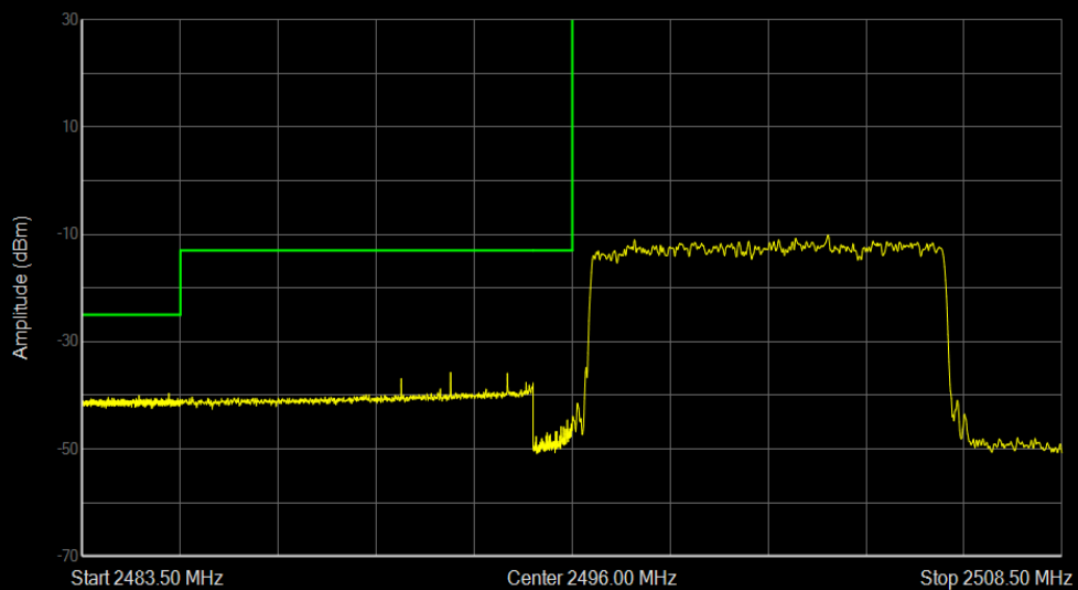
Band41 QAM16 BW=10MHz Channel=39700 RB Size=50 Position=#0
