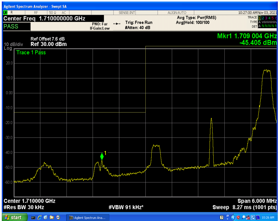
Band4 QAM16 BW=3MHz Channel=19965 RB Size=1 Position=#0
