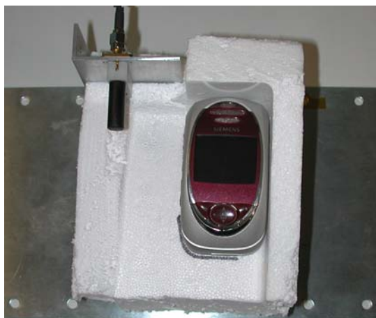
Fig. 8: Provided coupler to control the output power.
