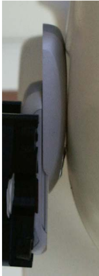
Fig. 37: Cheek position, right side, with slider up.
