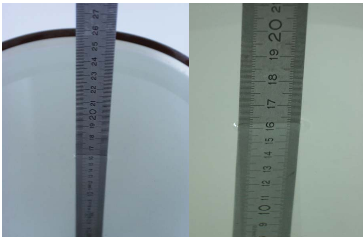
Fig. 52: Liquid depth for PCS 1900 Head and Body measurements.
