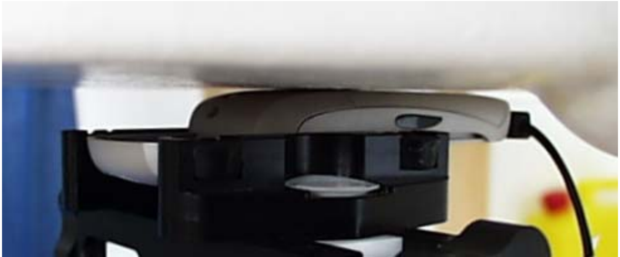
Fig. 47: Body worn configuration, slider up with headset, display towards the ground.
