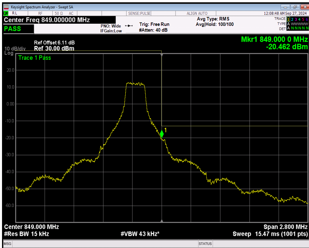
Band5 16QAM BW=1.4MHz Channel=20643 RB Size=6 Position=#0
