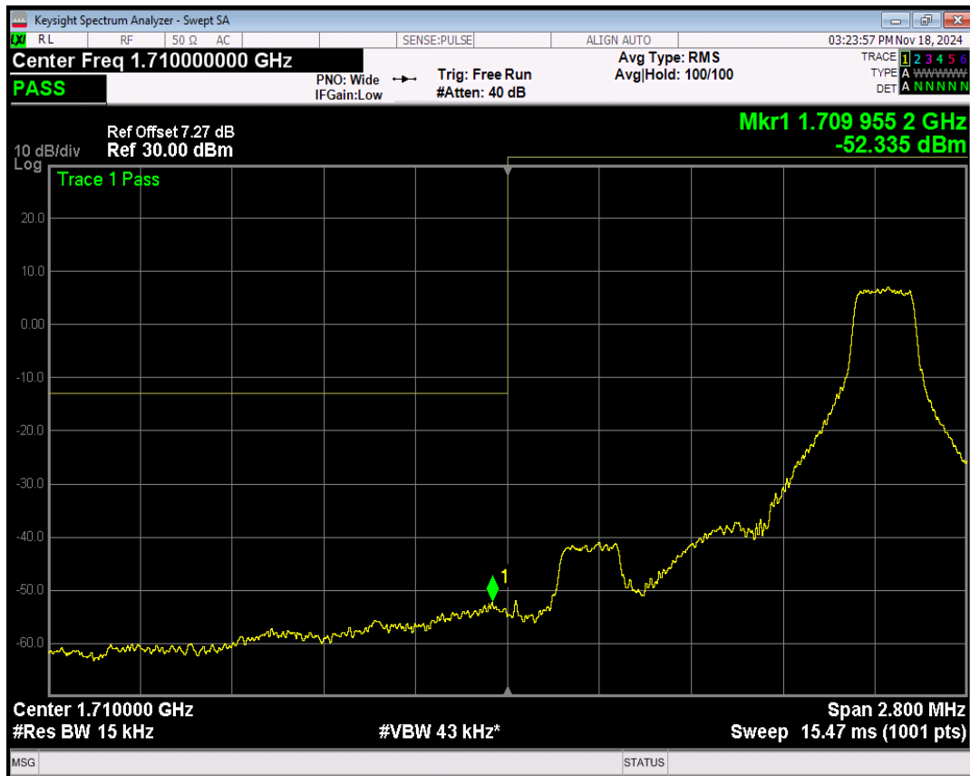
Band66 16QAM BW=1.4MHz Channel=131979 RB Size=6 Position=#0
