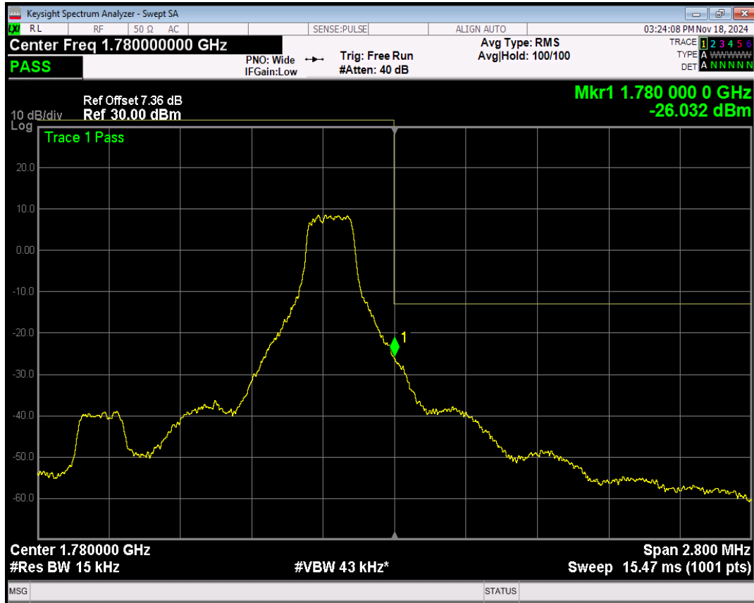
Band66 QPSK BW=1.4MHz Channel=132665 RB Size=6 Position=#0
