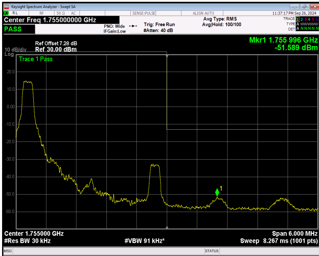
Band4 16QAM BW=3MHz Channel=20385 RB Size=1 Position=#Max
