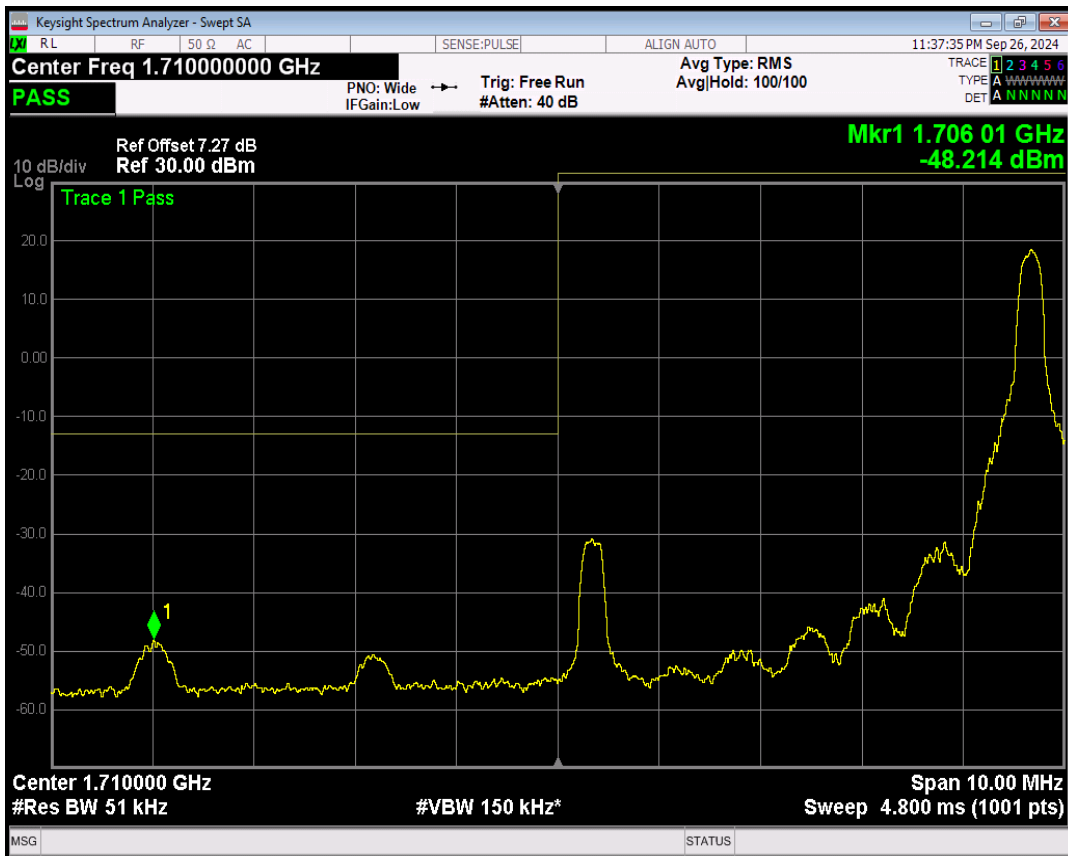
Band4 16QAM BW=5MHz Channel=19975 RB Size=25 Position=#0
