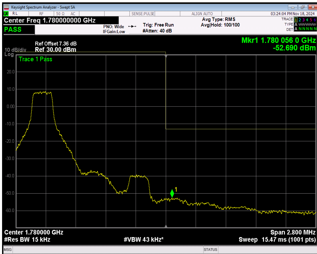
Band66 QPSK BW=1.4MHz Channel=132665 RB Size=1 Position=#Max
