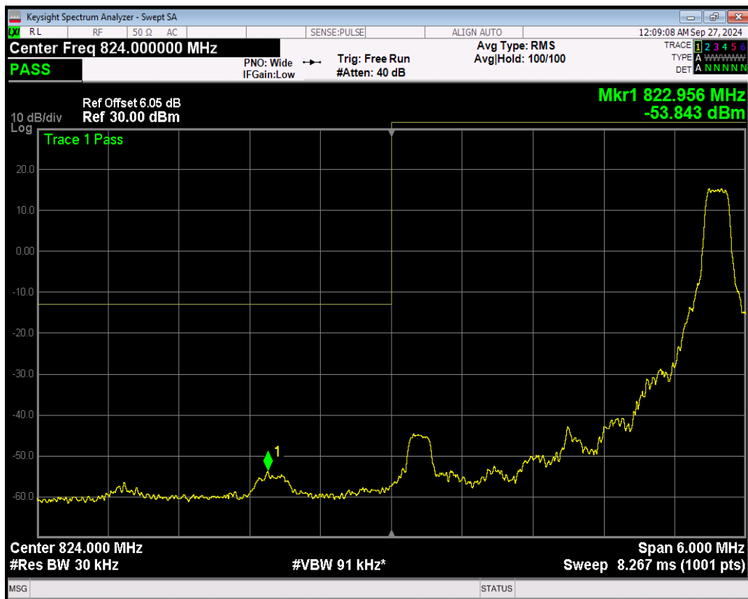
Band5 16QAM BW=3MHz Channel=20415 RB Size=15 Position=#0
