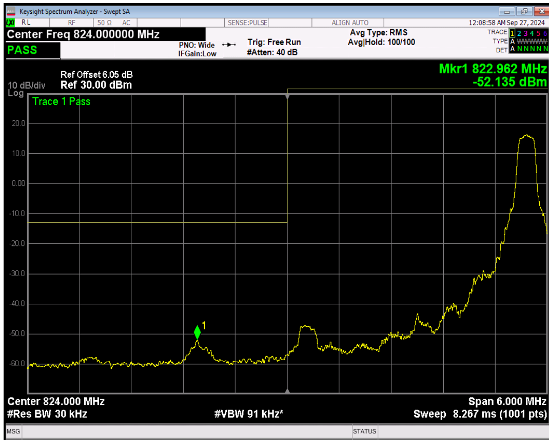
Band5 QPSK BW=3MHz Channel=20415 RB Size=15 Position=#0
