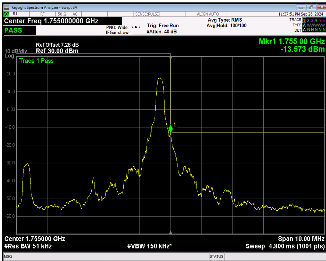
Band4 16QAM BW=5MHz Channel=20375 RB Size=25 Position=#0
