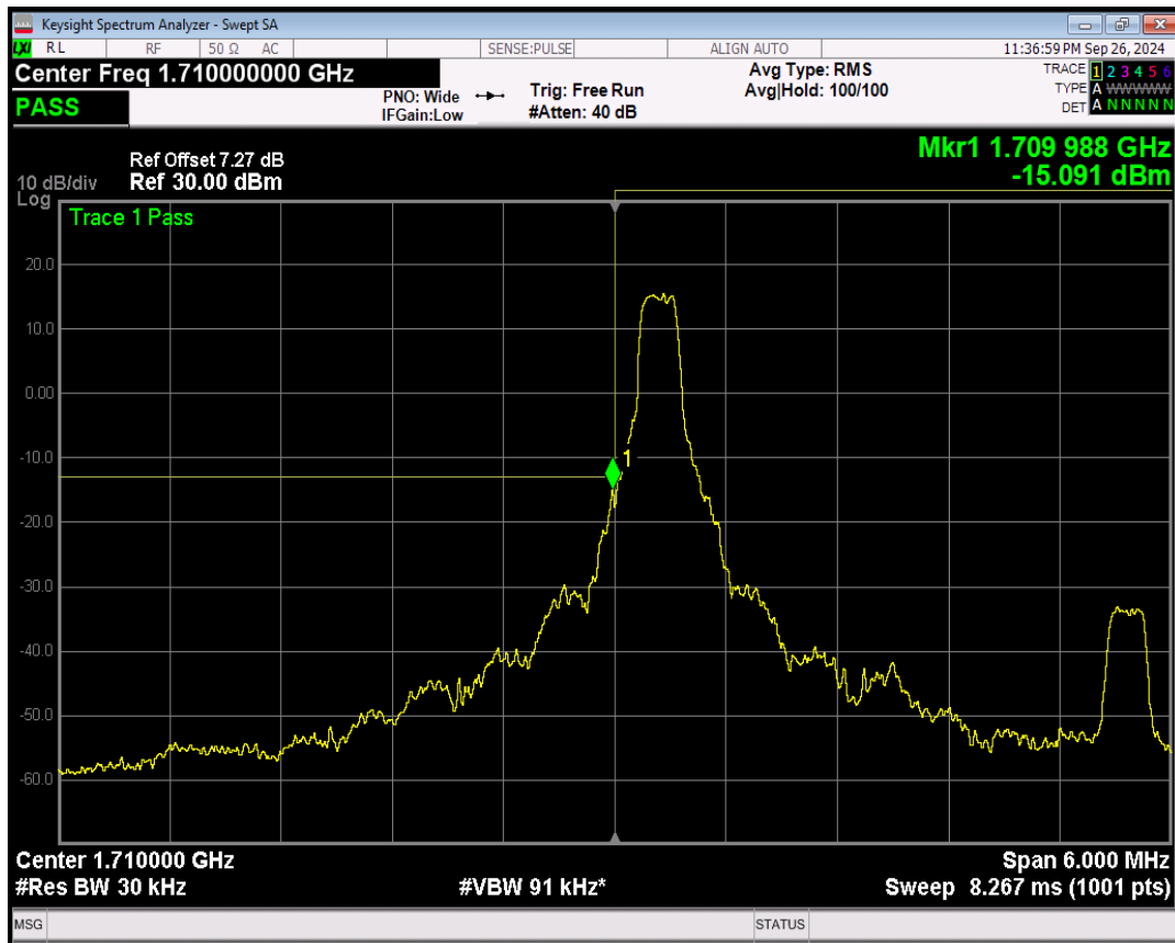
Band4 16QAM BW=3MHz Channel=19965 RB Size=1 Position=#Max
