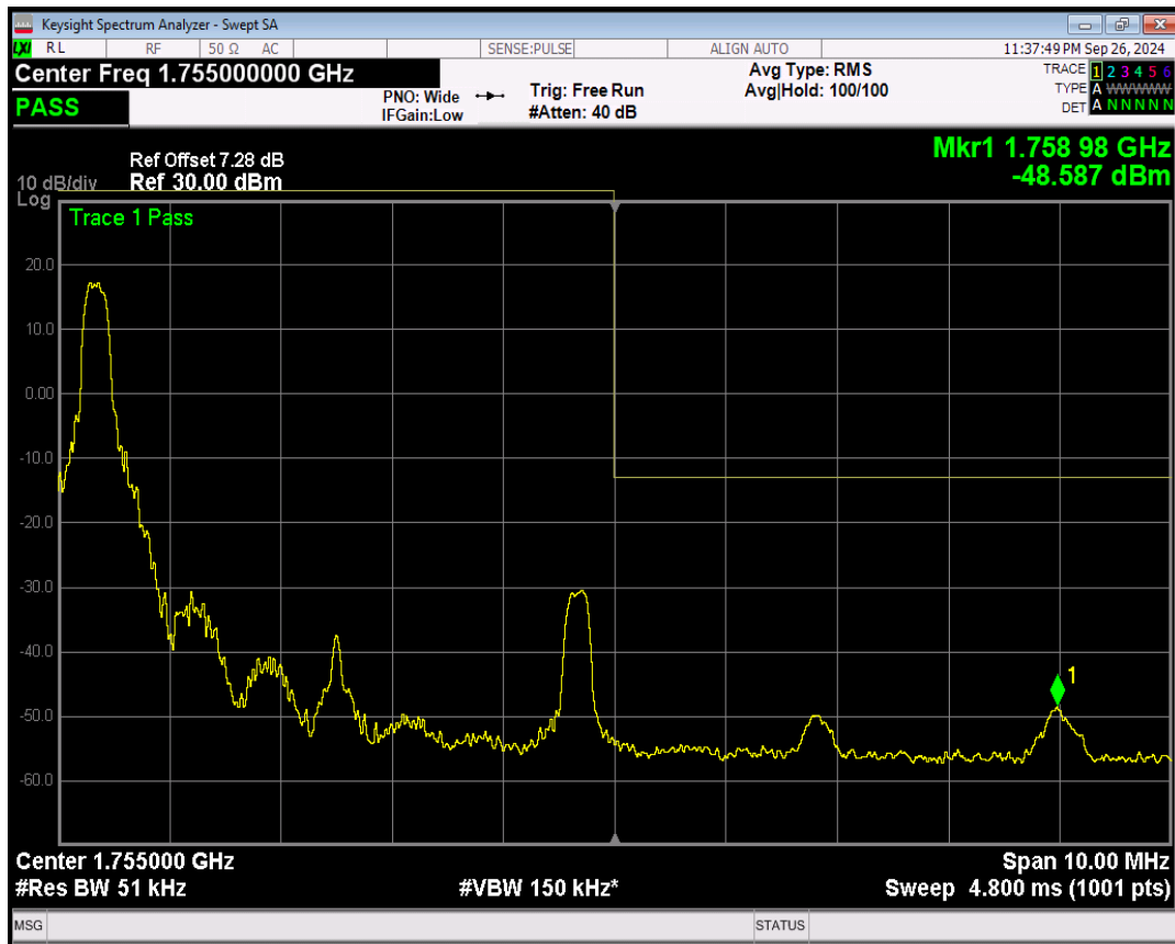
Band4 16QAM BW=5MHz Channel=20375 RB Size=1 Position=#Max
