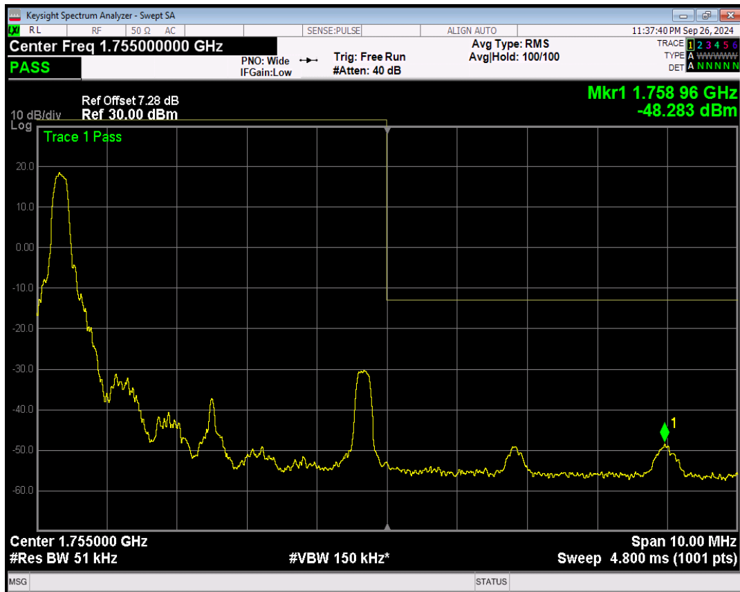
Band4 QPSK BW=5MHz Channel=20375 RB Size=1 Position=#Max
