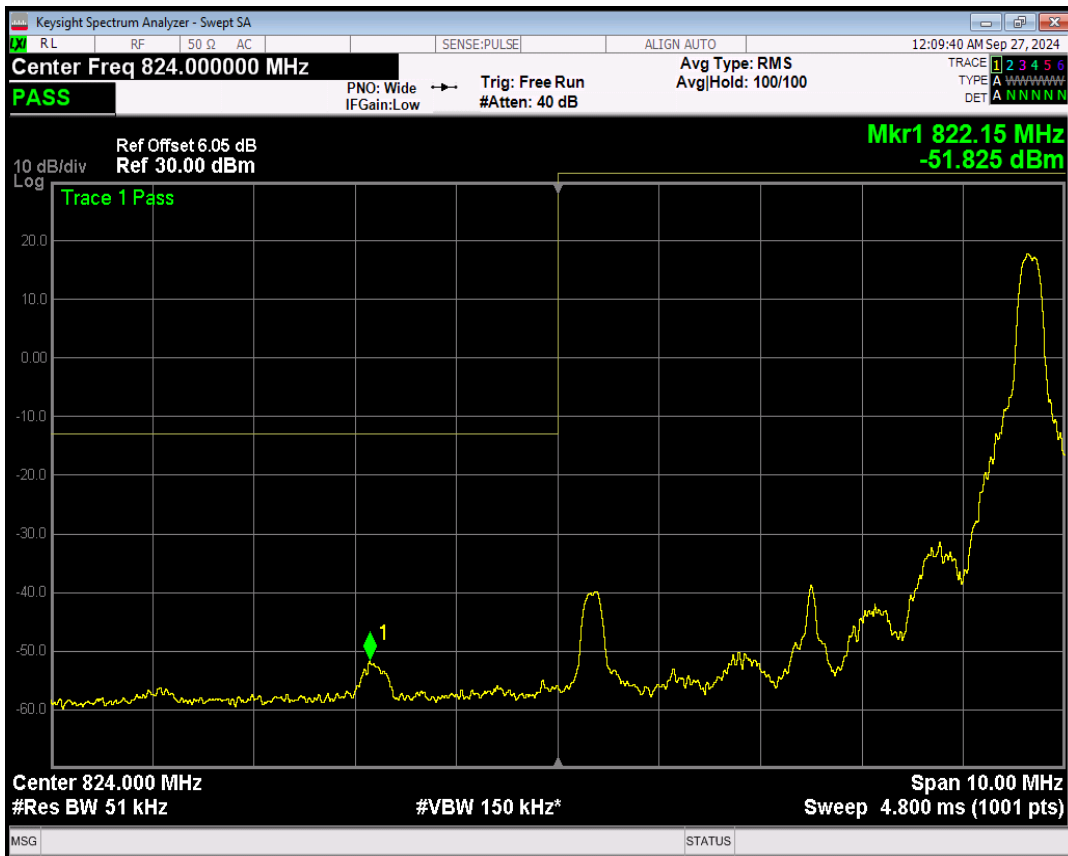
Band5 16QAM BW=5MHz Channel=20425 RB Size=25 Position=#0
