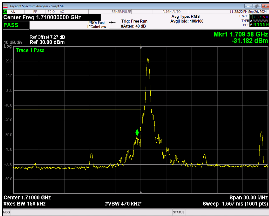
Band4 QPSK BW=15MHz Channel=20025 RB Size=1 Position=#Max
