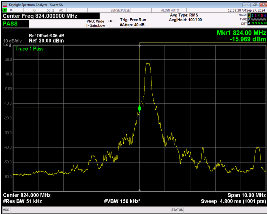
Band5 16QAM BW=5MHz Channel=20425 RB Size=1 Position=#Max
