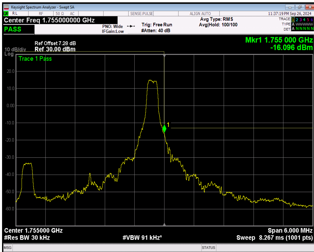
Band4 16QAM BW=3MHz Channel=20385 RB Size=15 Position=#0
