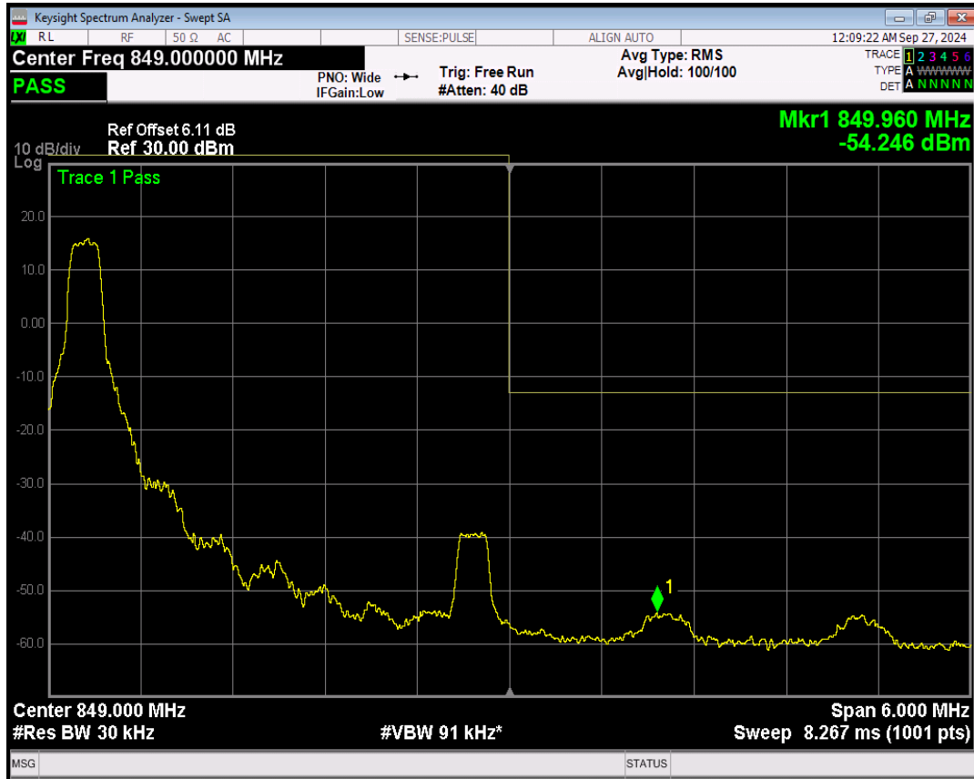
Band5 16QAM BW=3MHz Channel=20635 RB Size=1 Position=#Max
