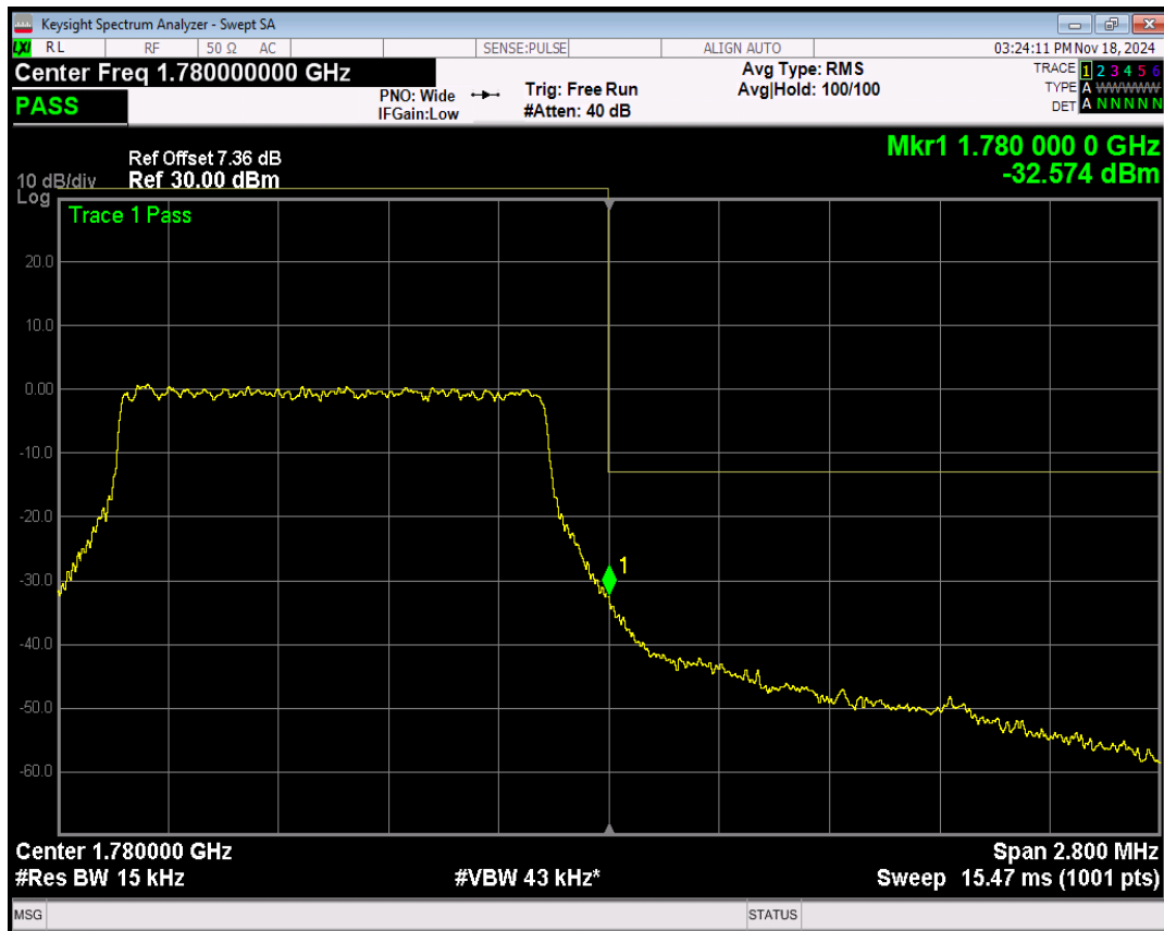
Band66 16QAM BW=1.4MHz Channel=132665 RB Size=1 Position=#0
