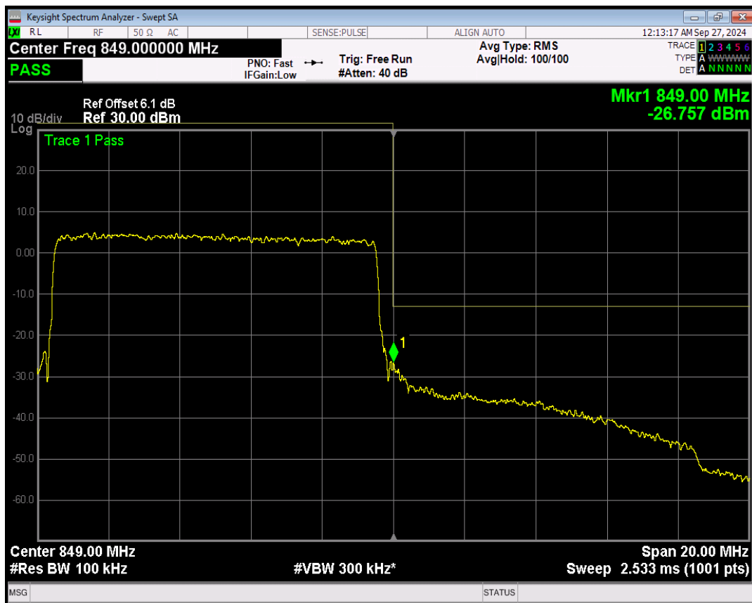
Band5 16QAM BW=10MHz Channel=20600 RB Size=1 Position=#0
