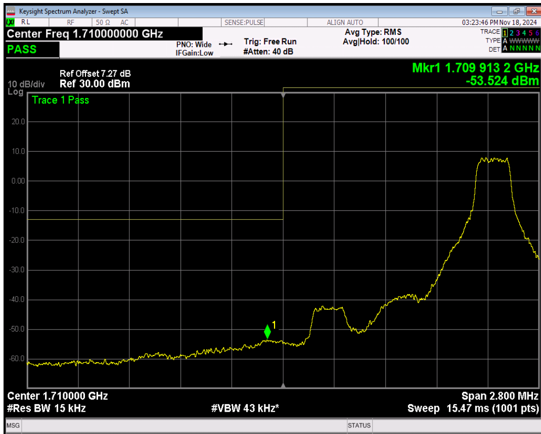
Band66 QPSK BW=1.4MHz Channel=131979 RB Size=6 Position=#0
