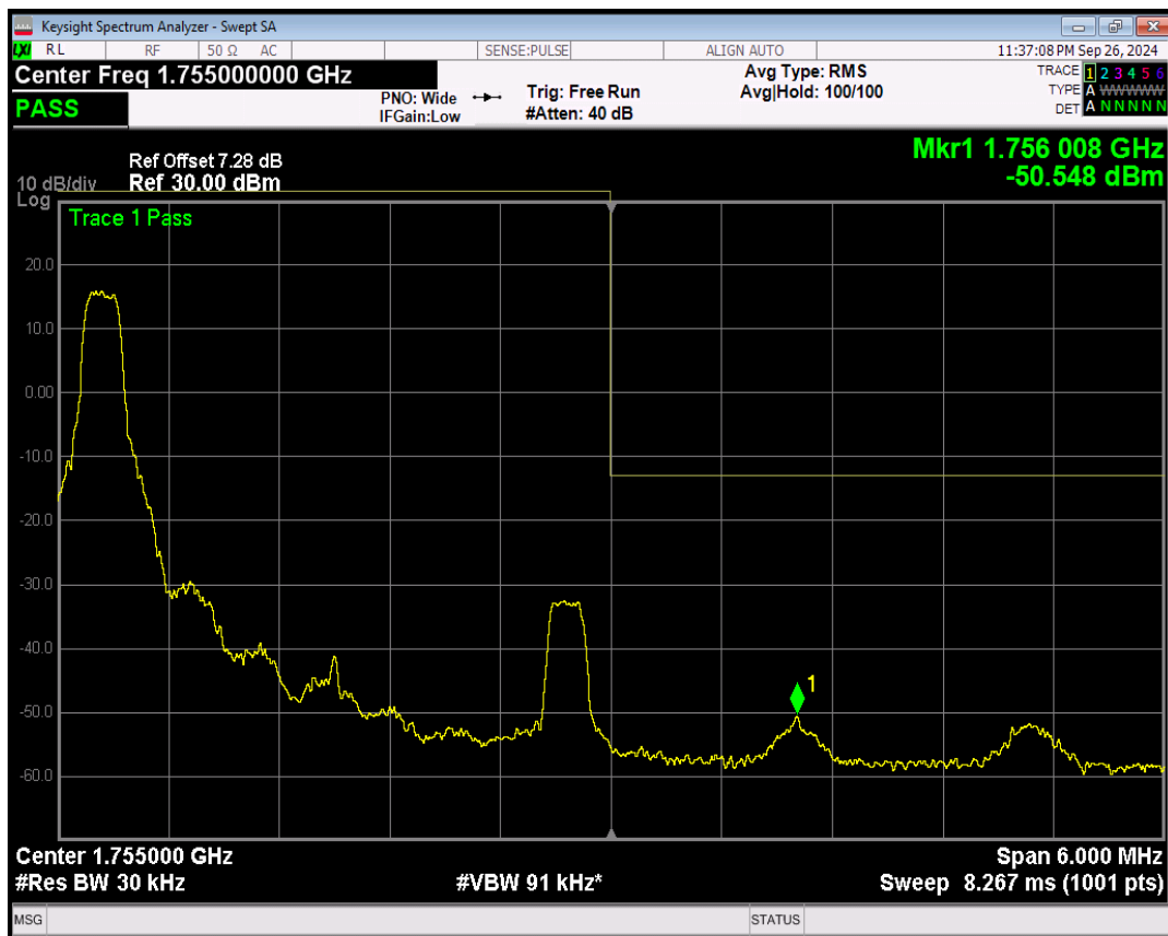
Band4 QPSK BW=3MHz Channel=20385 RB Size=1 Position=#Max
