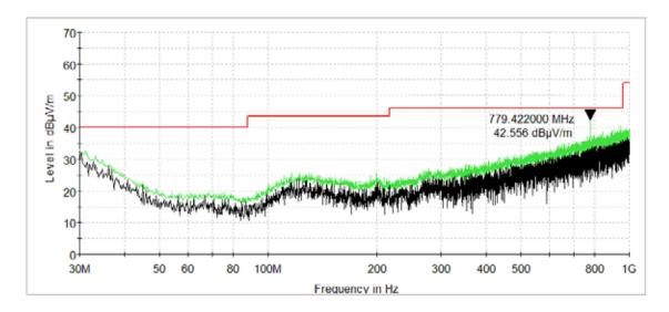
13 MHz: Characterization Scan, 30 MHz to 1000 MHz, Vertical
