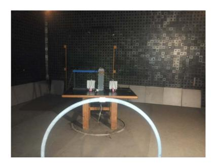
Photograph No.8 Spurious emissions measurement setup in the anechoic chamber in 30 -1000 MHz
