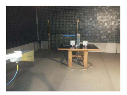
Photograph No.10 Spurious emissions measurement setup in the anechoic chamber, EUT close view
