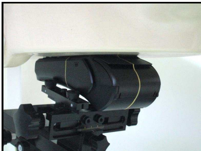
Front Face of EUT with 0 cm Gap (Body-Worn Mode)
