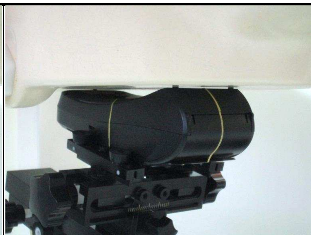
Rear Face of EUT with 0 cm Gap (Body-Worn Mode)
