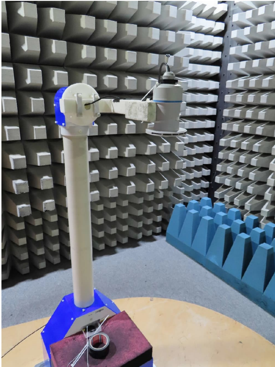
Test setup fully anechoic chamber with EUT 2A (1 GHz - 40 GHz)
