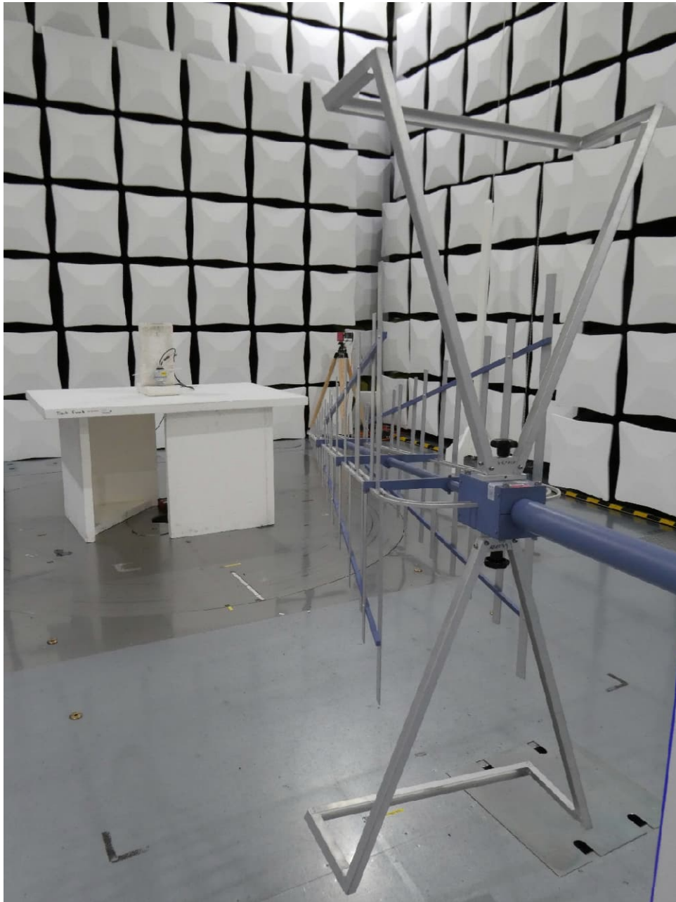
Test setup semi anechoic chamber with EUT 1A (<1 GHz, position 2)
