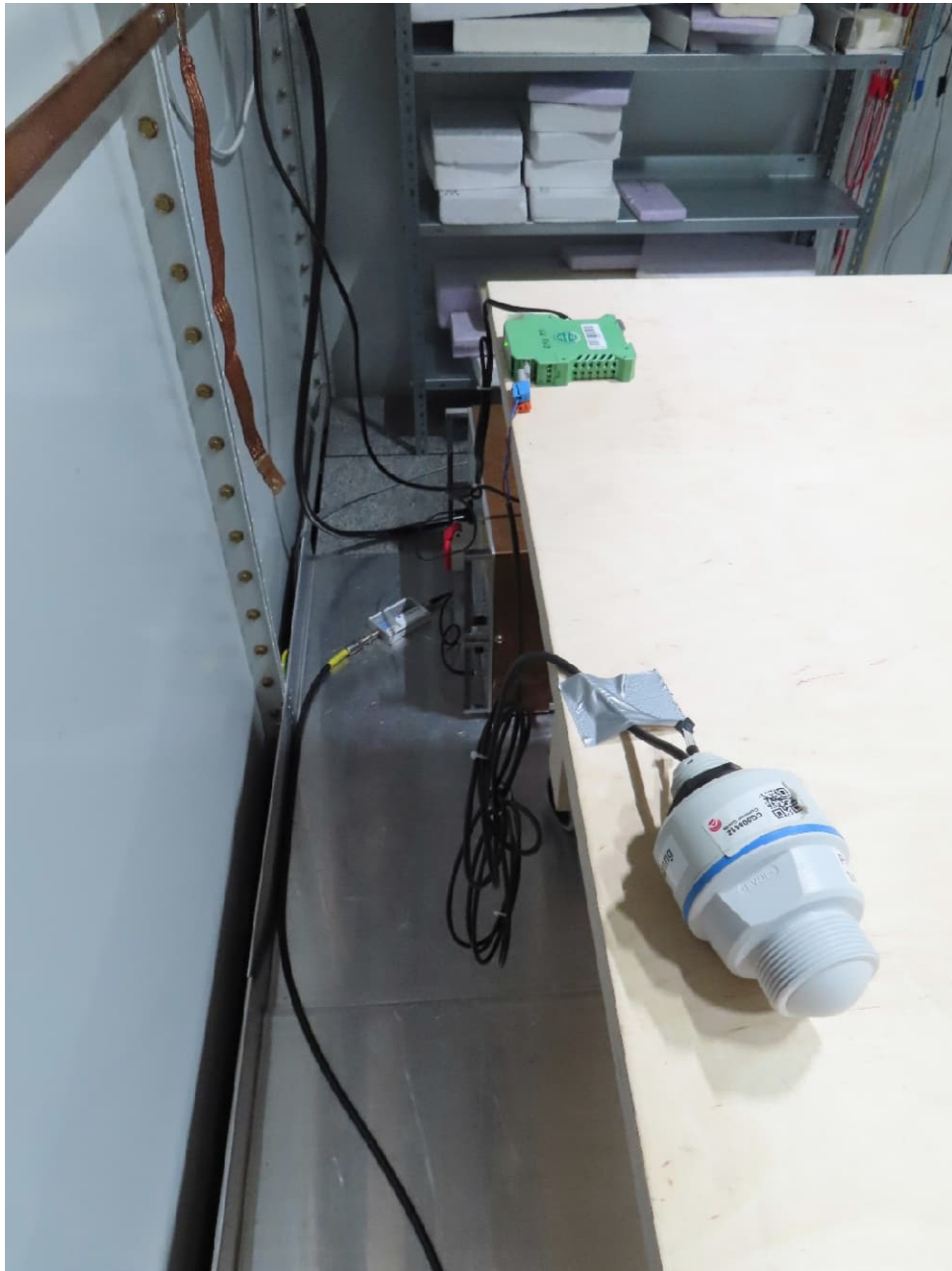
Test AC power line conducted emissions with EUT 1A
