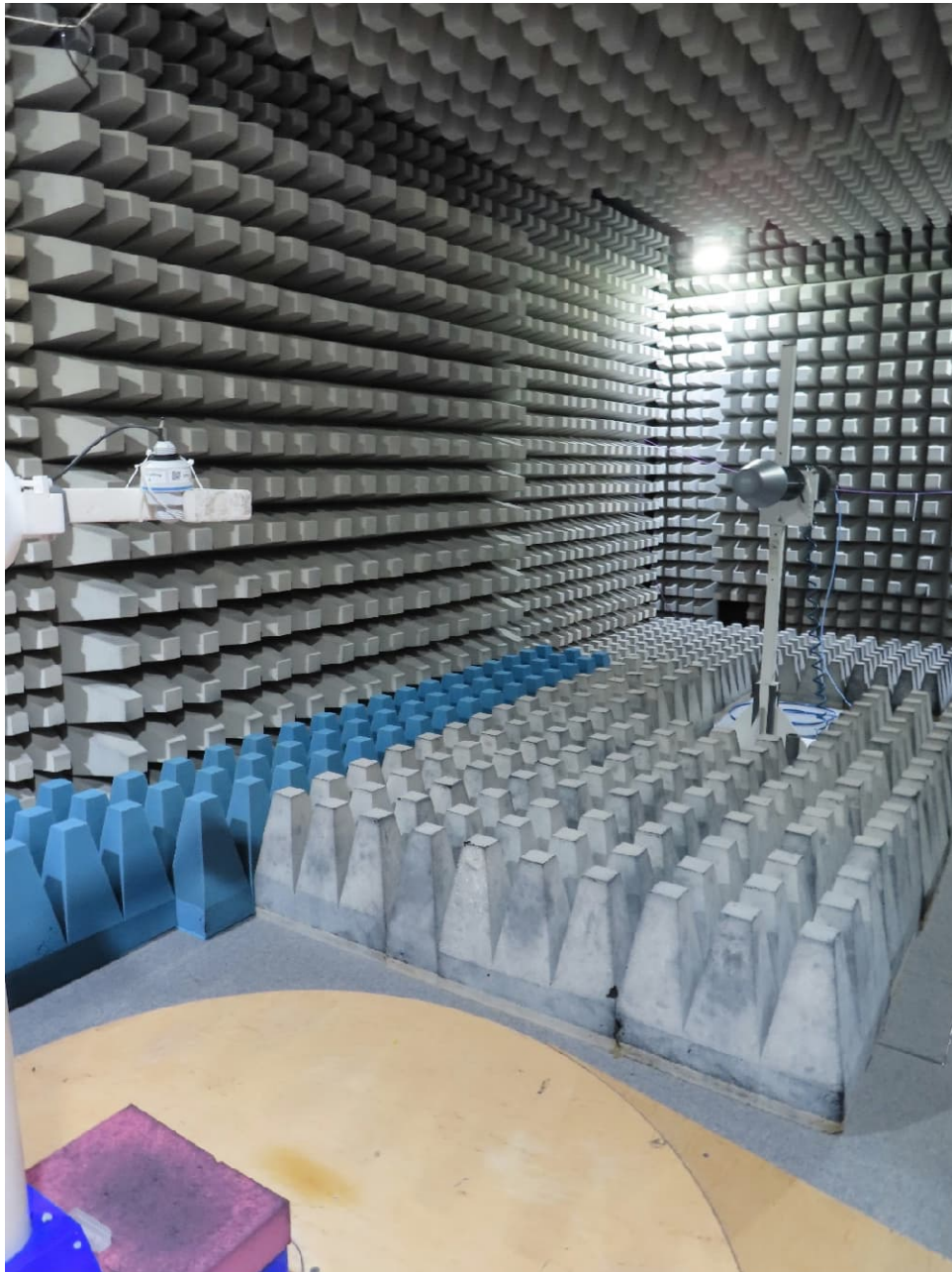
Test setup fully anechoic chamber with EUT 1A (1 GHz – 12 GHz)
