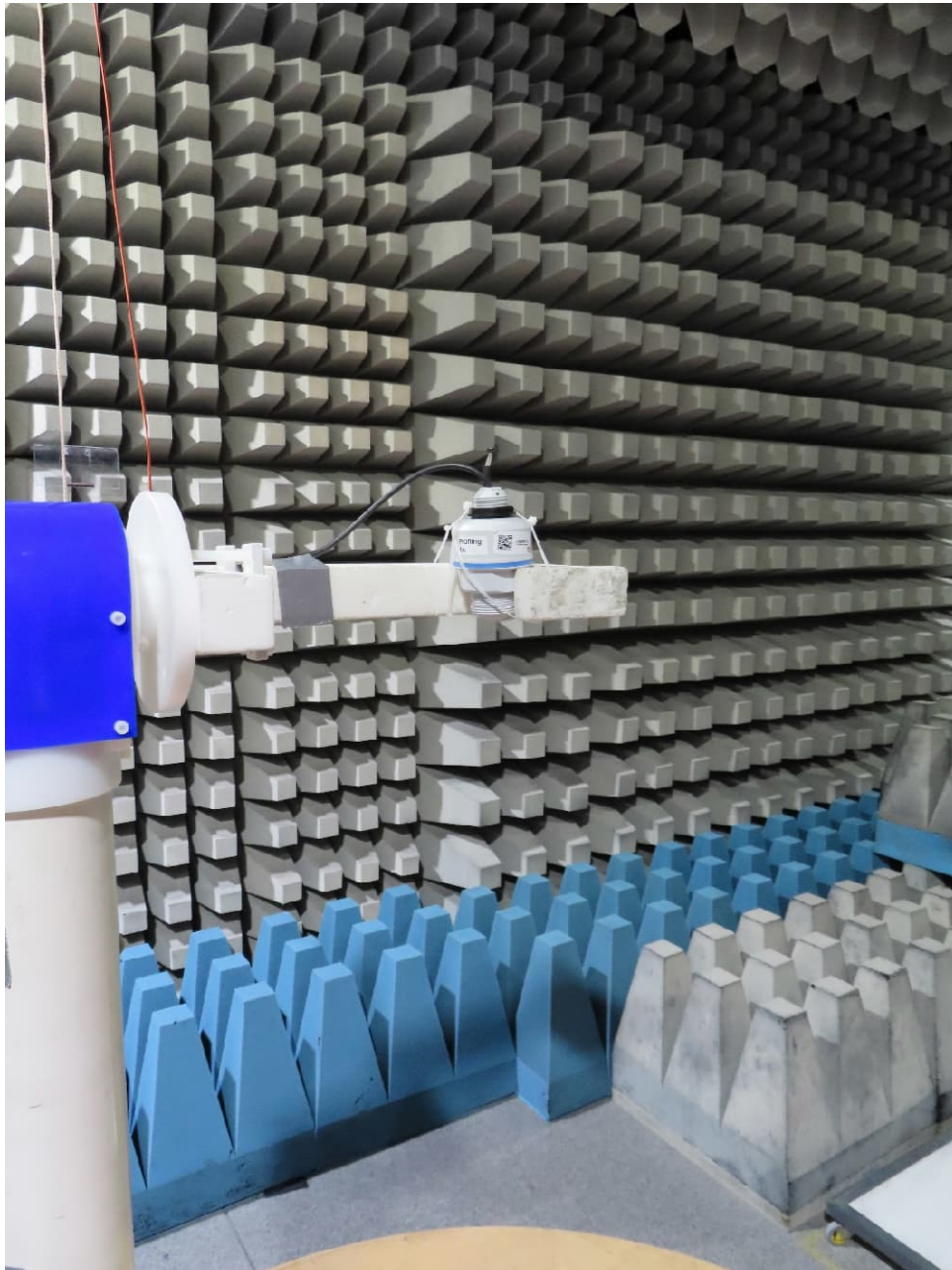
Test setup fully anechoic chamber with EUT 1A (1 GHz - 40 GHz)
