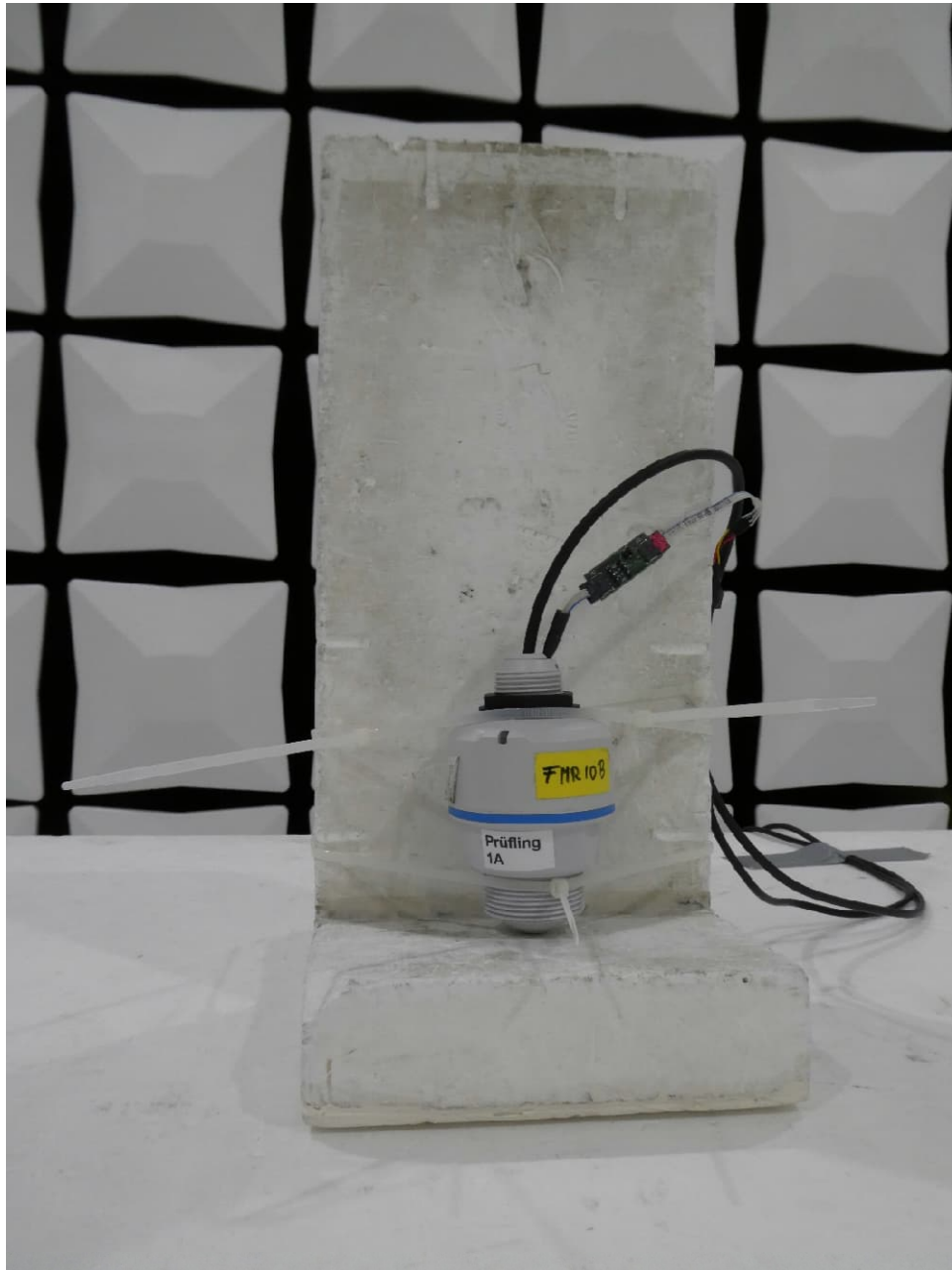
Test setup semi anechoic chamber with EUT 1A (position 2)
