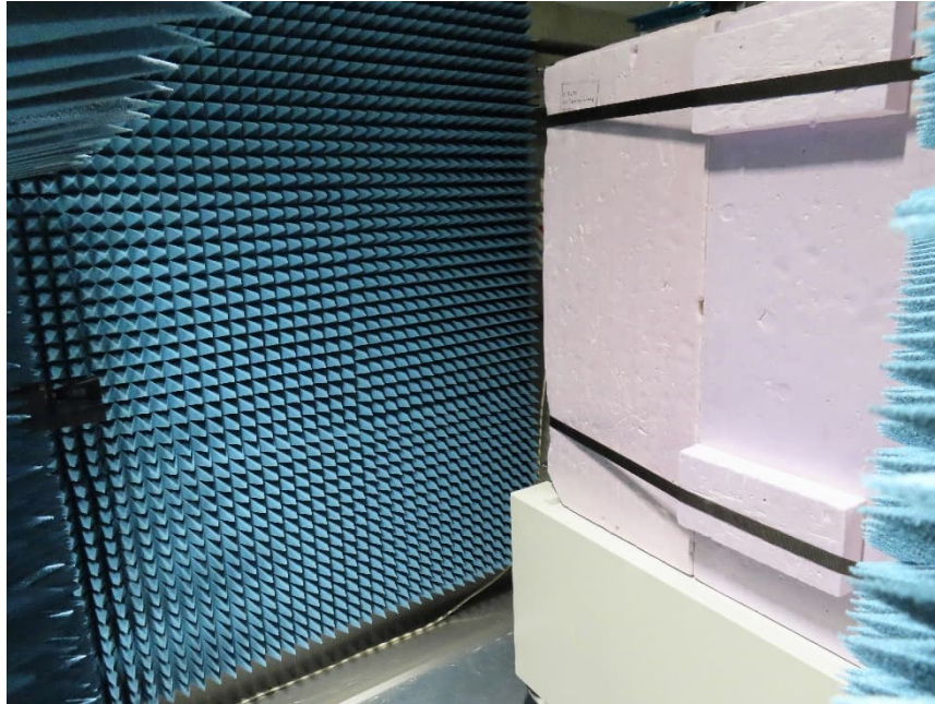
Test temperature chamber with EUT 2A (with isolation)
