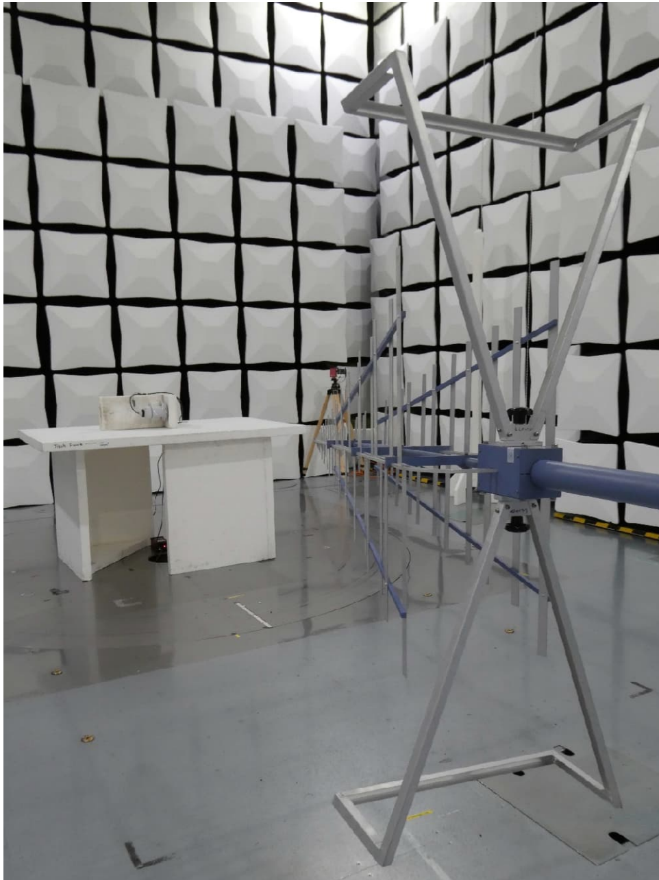
Test setup semi anechoic chamber with EUT 2A (<1 GHz, position 1)
