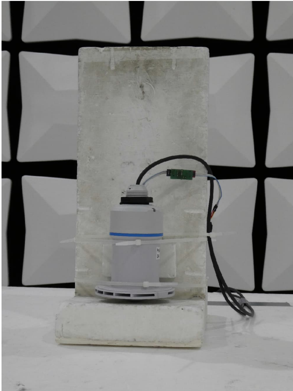
Test setup semi anechoic chamber with EUT 2A (position 2)
