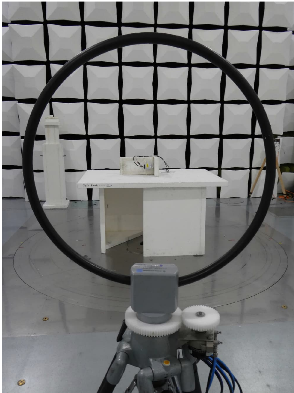
Test setup semi anechoic chamber with EUT 1A (<30 MHz, position 1)
