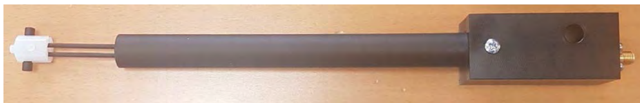
Figure 1 – MVG COMOSAR Validation Dipole
