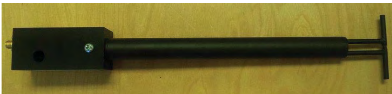
Figure 1 – MVG COMOSAR Validation Dipole
