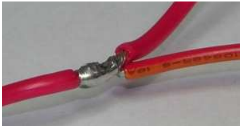
Figure 5: Correctly Soldered Connection
