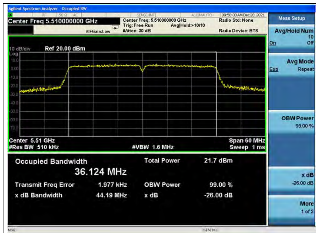
(Channel 102, 5510MHz, 802.11ac (VHT40))
