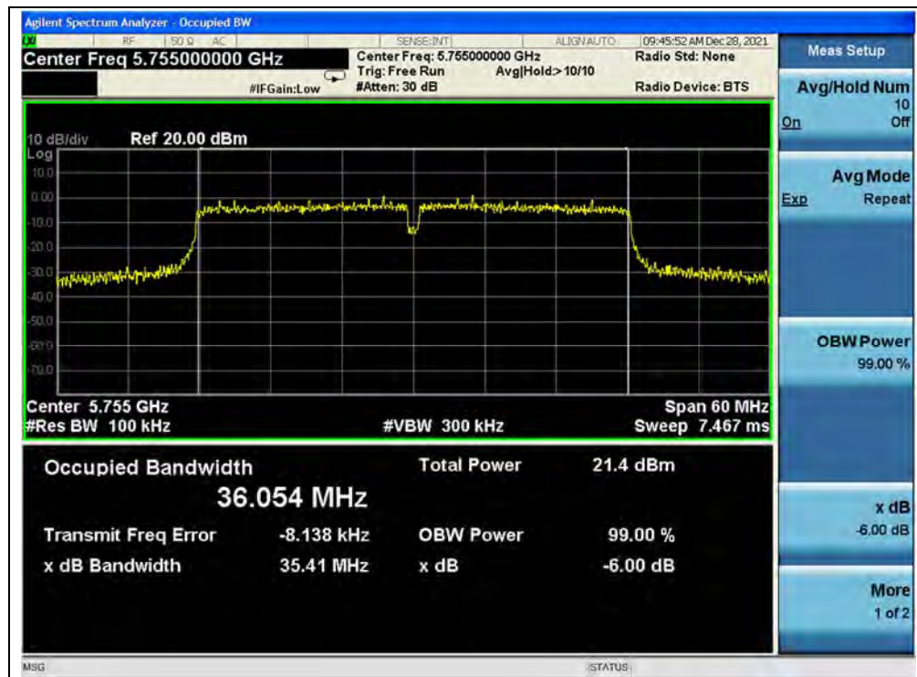
(Channel 151, 5755MHz, 802.11ac (VHT40))
