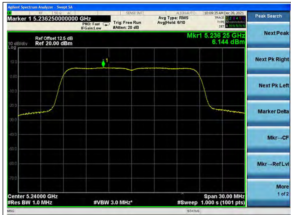
(Channel 48, 5240MHz, 802.11ac (VHT20))
