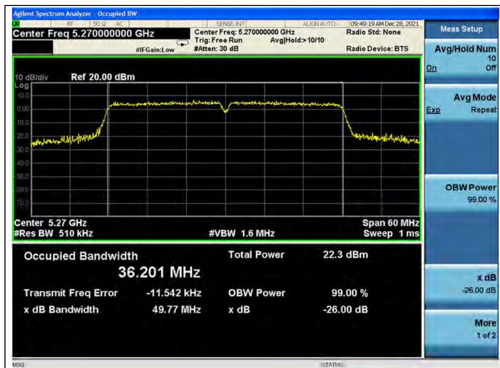
(Channel 54, 5270MHz, 802.11ac (VHT40))
