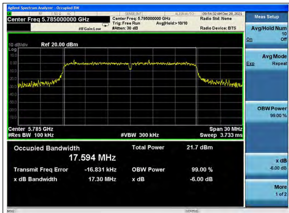
(Channel 157, 5785MHz, 802.11 ac (VHT20))
