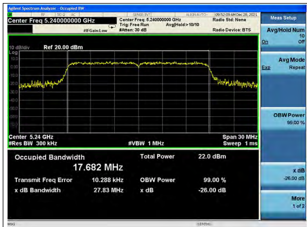
(Channel 48, 5240MHz, 802.11ac (VHT20))
