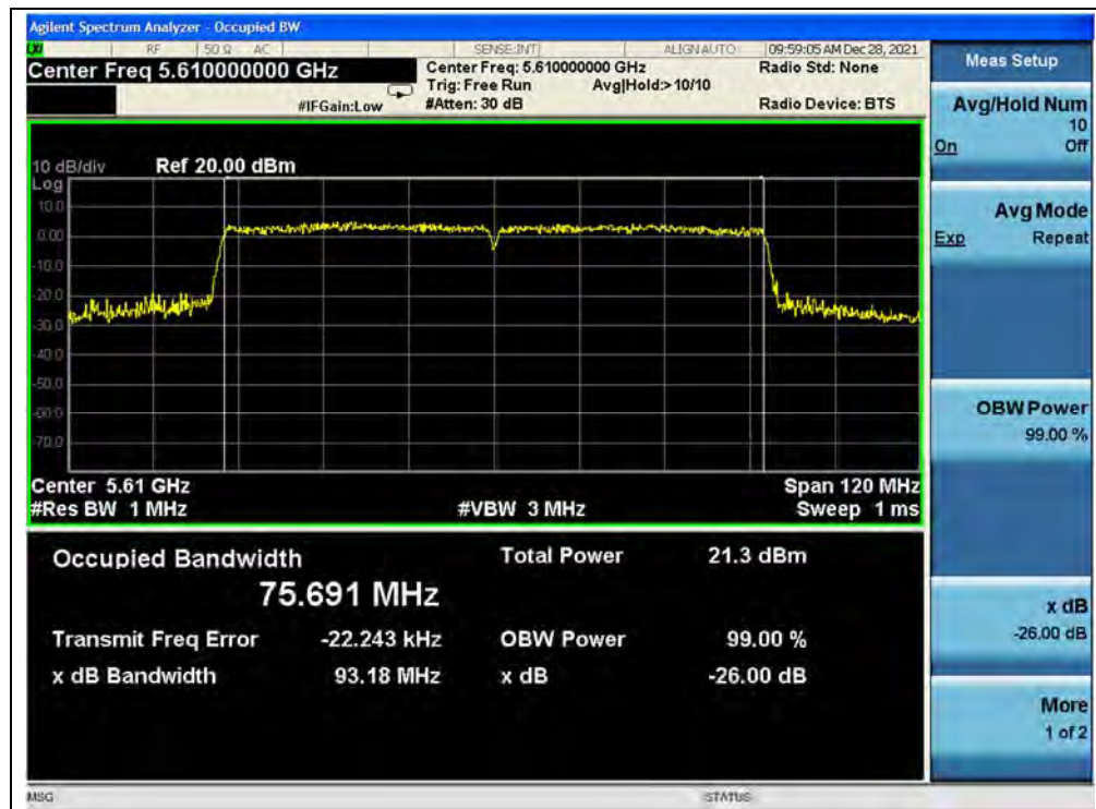
(Channel 122, 5610MHz, 802.11ac (VHT80))
