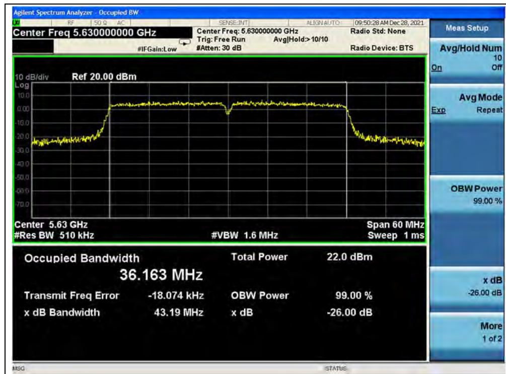
(Channel 126, 5630MHz, 802.11ac (VHT40))
