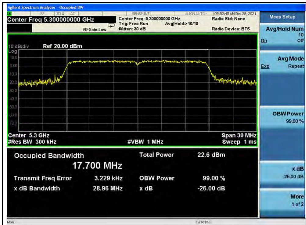
(Channel 60, 5300MHz, 802.11ac (VHT20))
