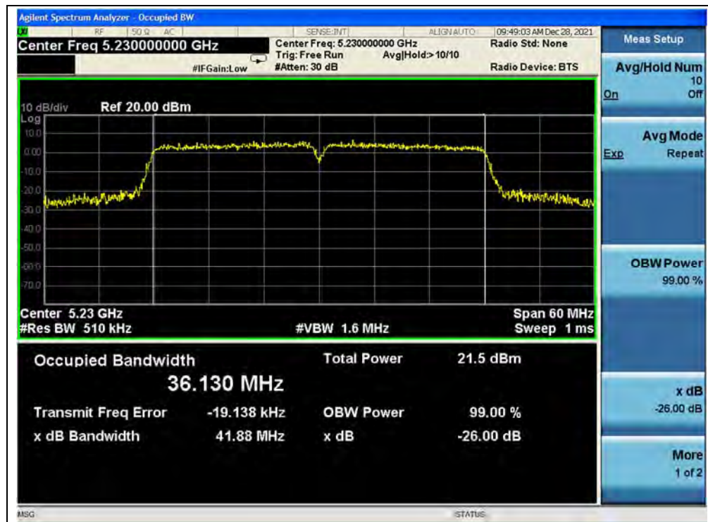
(Channel 46, 5230MHz, 802.11ac (VHT40))
