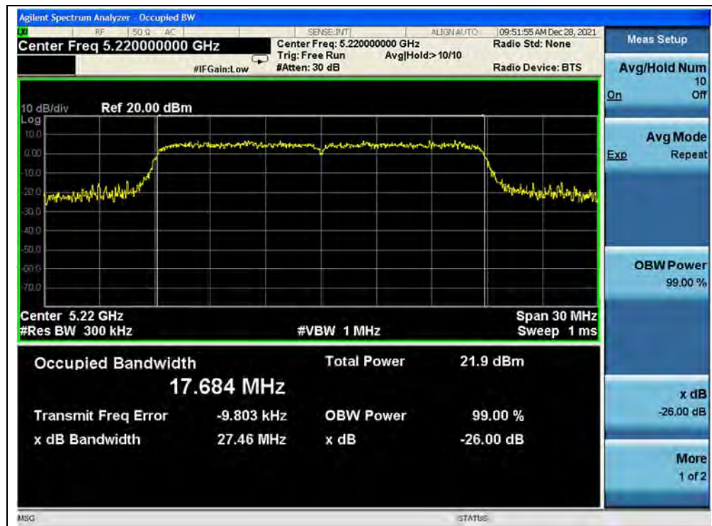
(Channel 44, 5220MHz, 802.11ac (VHT20))
