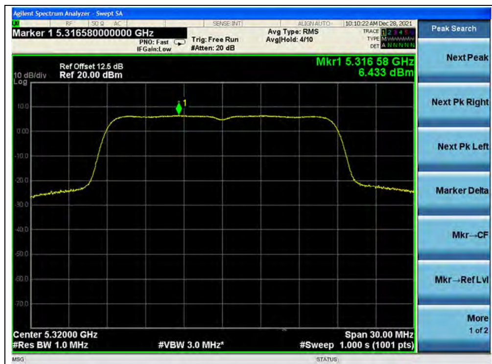
(Channel 64, 5320MHz, 802.11ac (VHT20))
