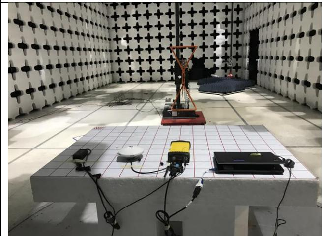
Radiated Emissions below 1GHz – Front View
