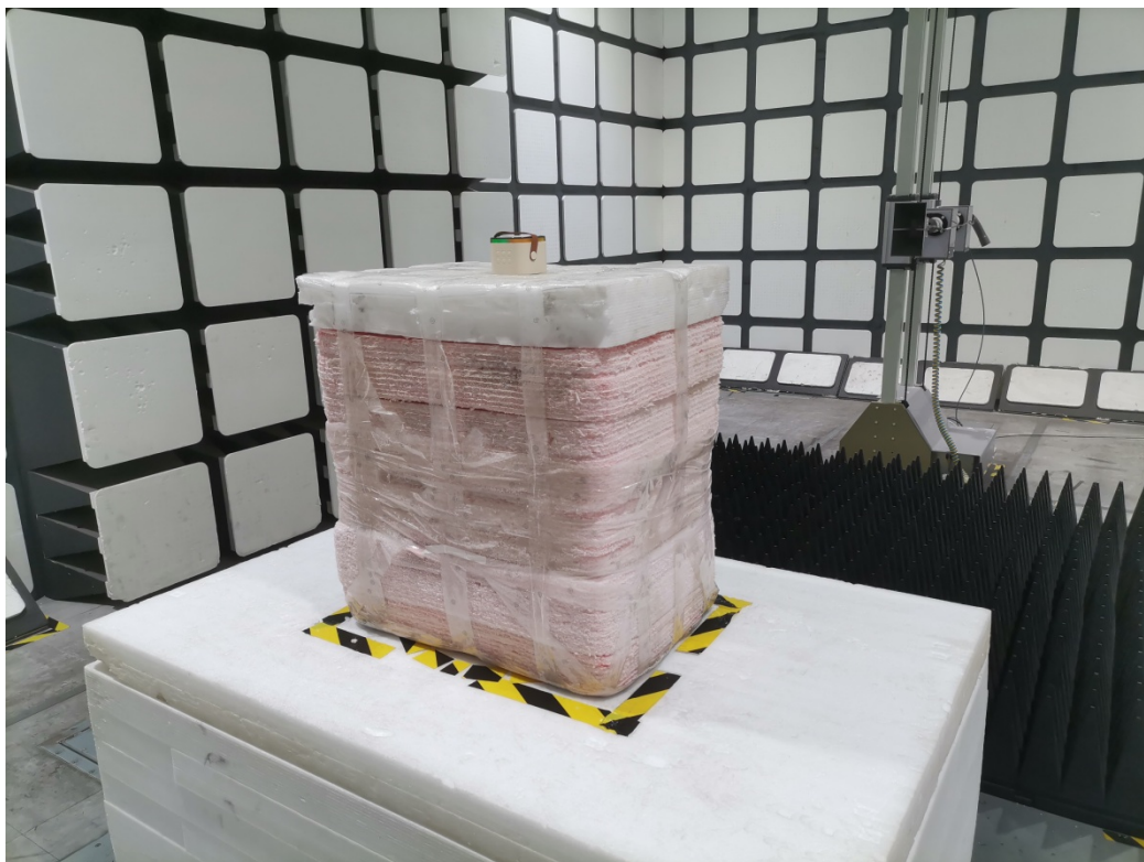
Radiated Emissions View (1-18 GHz)
