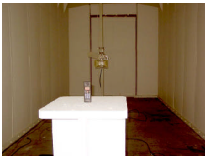
Uniden - Handset Testing Peak Power Spectral Density - Radiated
