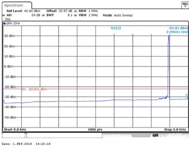
Figure 57 Spurious Emissions (9kHz – 3GHz) – 16QAM (2593.0 MHz) (20MHz Channel BW)
