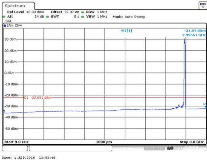
Figure 129 Spurious Emissions (9kHz – 3GHz) – 16QAM (2593.0 MHz) (20MHz Channel BW)
