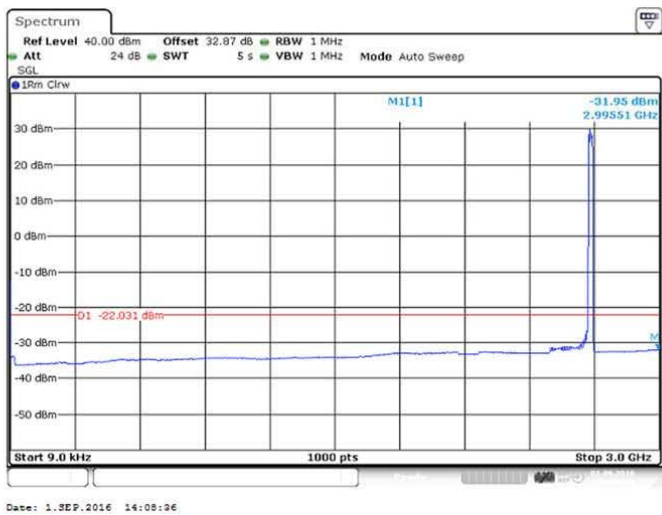
Figure 148 Spurious Emissions (9kHz – 3GHz) – 64QAM (2593.0 MHz) (20MHz Channel BW)
