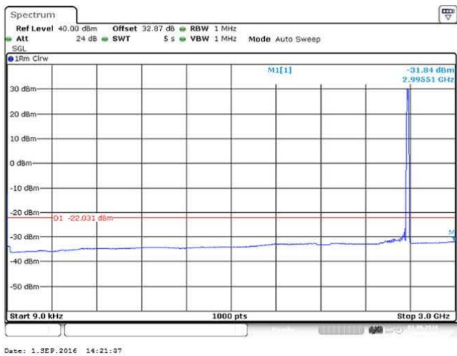
Figure 53 Spurious Emissions (9kHz – 3GHz) – 64QAM (2593.0 MHz) (20MHz Channel BW)
