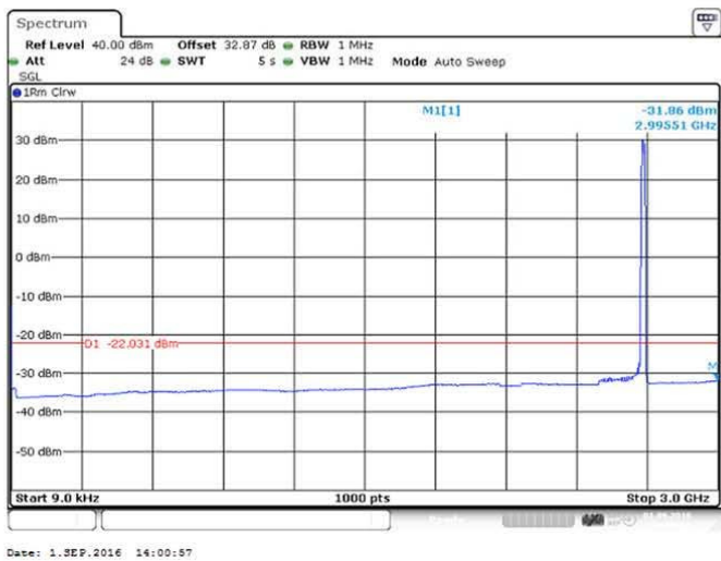
Figure 136 Spurious Emissions (9kHz – 3GHz) – 64QAM (2593.0 MHz) (20MHz Channel BW)
