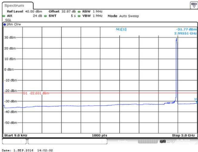
Figure 140 Spurious Emissions (9kHz – 3GHz) – 16QAM (2593.0 MHz) (20MHz Channel BW)
