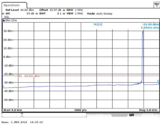
Figure 49 Spurious Emissions (9kHz – 3GHz) – QPSK (2593.0 MHz) (20MHz Channel BW)
