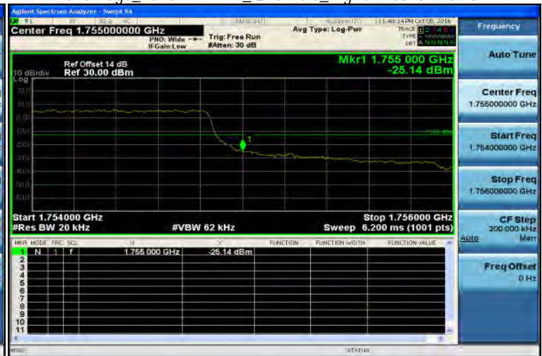
Band Edge_Band4 1.4MHz_QPSK 6 0_HighCH20393-1754.3
