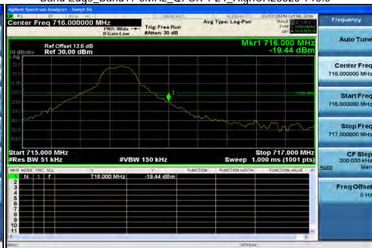
Band Edge_Band17 5MHz_QPSK 1 24_HighCH23825-713.5
