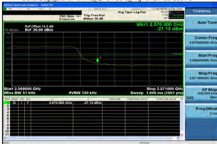
Band Edge_Band7 5MHz_QPSK 25 0_HighCH21425-2567.5
