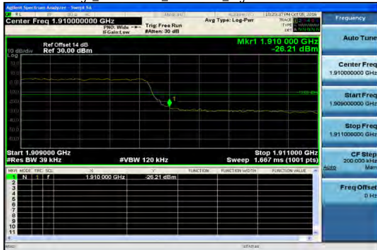
Band Edge_Band2 3MHz_QPSK 15 0_HighCH19185-1908.5
