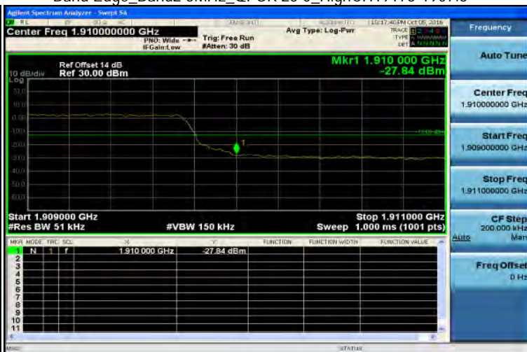
Band Edge_Band2 5MHz_QPSK 25 0_HighCH19175-1907.5
