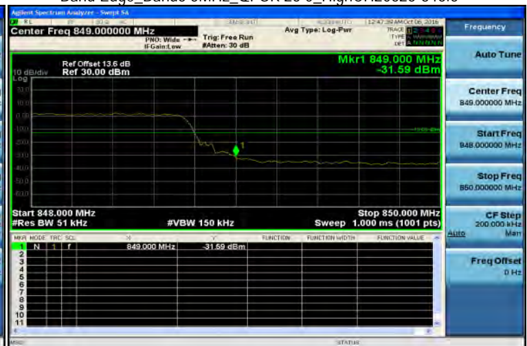
Band Edge_Band5 5MHz_QPSK 25 0_HighCH20625-846.5
