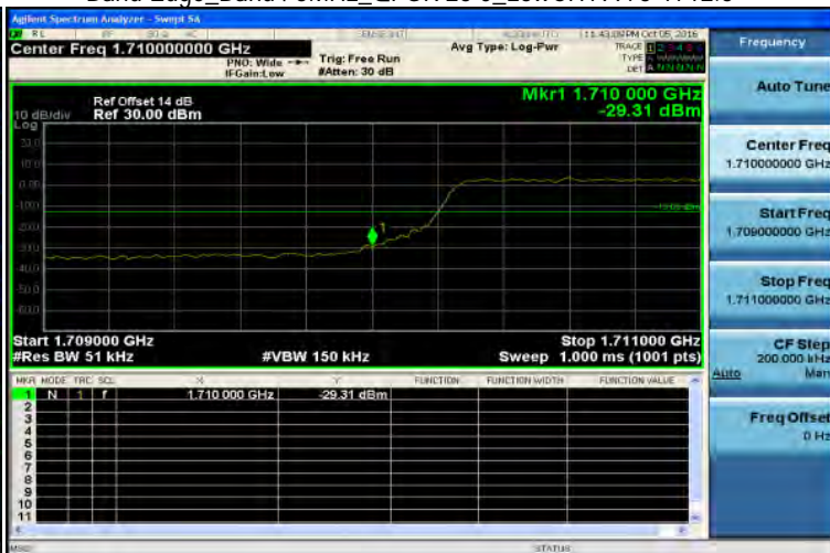
Band Edge_Band4 5MHz_QPSK 25 0_LowCH19975-1712.5
