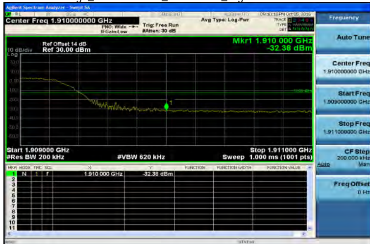
Band Edge_Band2 15MHz_QPSK 75 0_HighCH19125-1902.5
