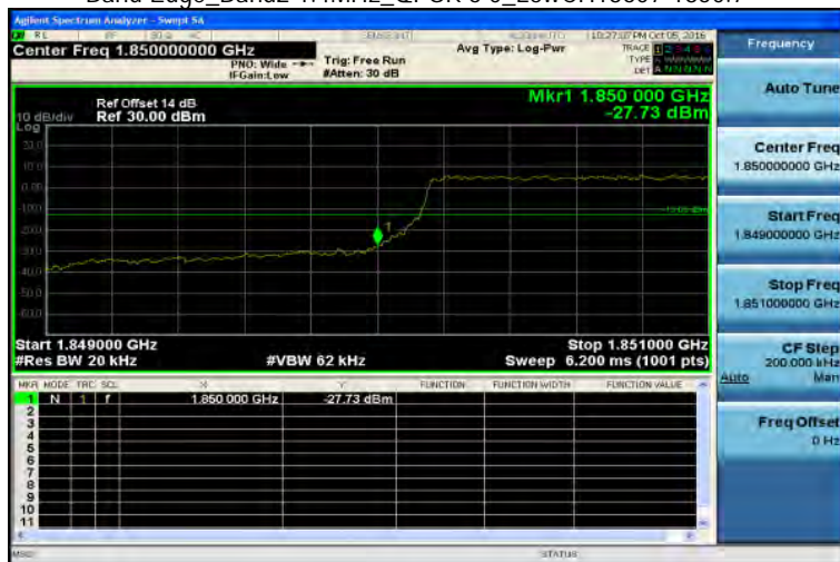
Band Edge_Band2 1.4MHz_QPSK 6 0_LowCH18607-1850.7
