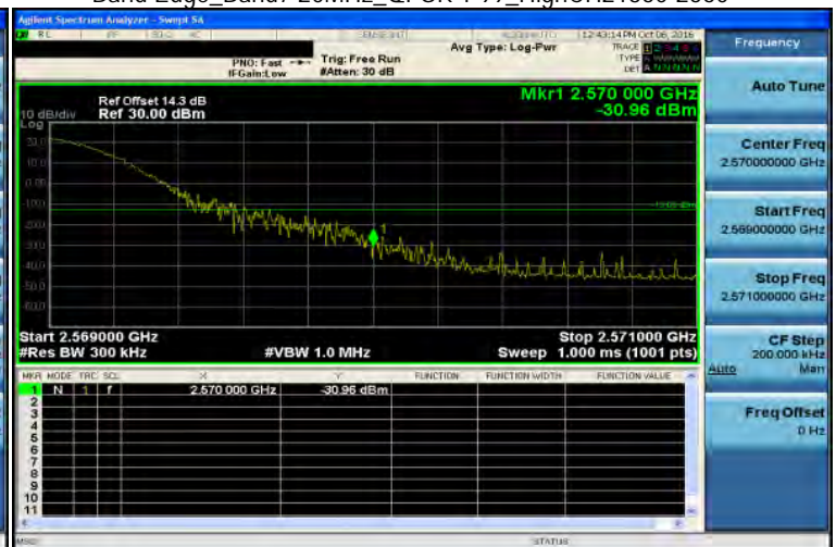
Band Edge_Band7 20MHz_QPSK 1 99_HighCH21350-2560
