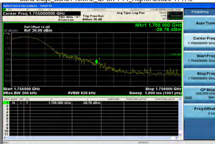
Band Edge_Band4 15MHz_QPSK 1 74_HighCH20325-1747.5
