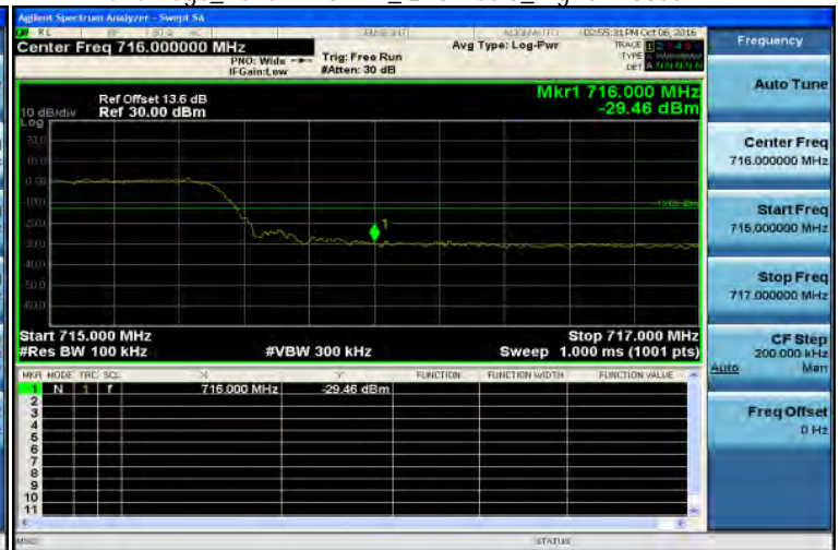
Band Edge_Band17 10MHz_QPSK 50 0_HighCH23800-711
