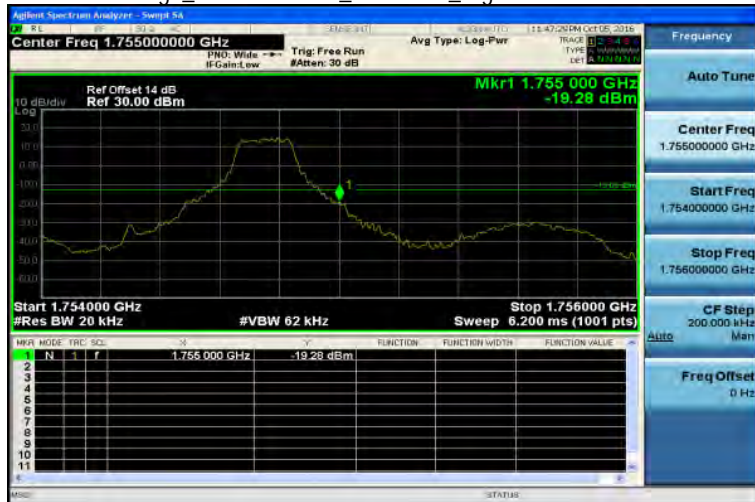
Band Edge_Band4 1.4MHz_QPSK 1 5_HighCH20393-1754.3
