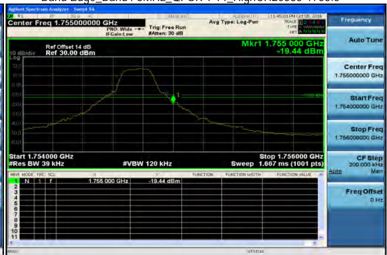
Band Edge_Band4 3MHz_QPSK 1 14_HighCH20385-1753.5
