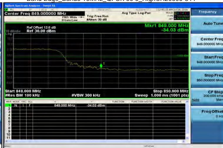
Band Edge_Band5 10MHz_QPSK 50 0_HighCH20600-844
