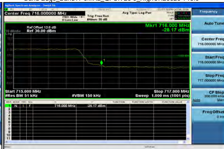
Band Edge_Band17 5MHz_QPSK 25 0_HighCH23825-713.5
