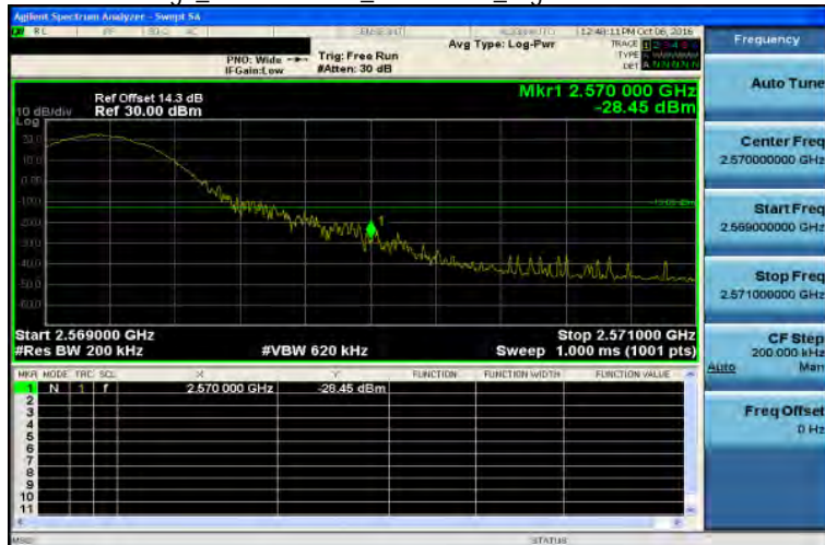
Band Edge_Band7 15MHz_QPSK 1 74_HighCH21375-2562.5
