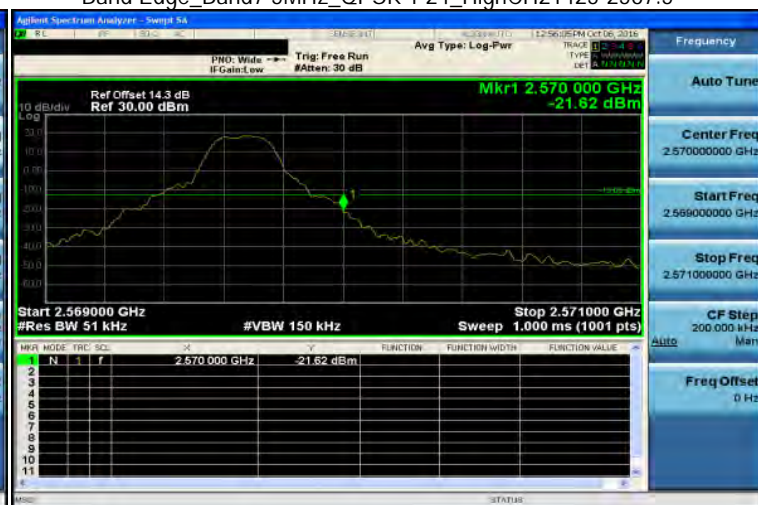
Band Edge_Band7 5MHz_QPSK 1 24_HighCH21425-2567.5
