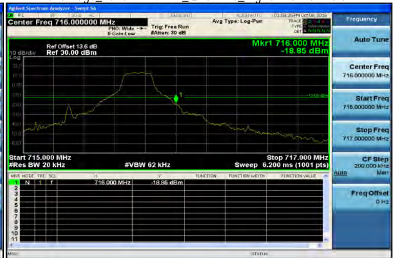
Band Edge_Band12 1.4MHz_QPSK 1 5_HighCH23173-715.3
