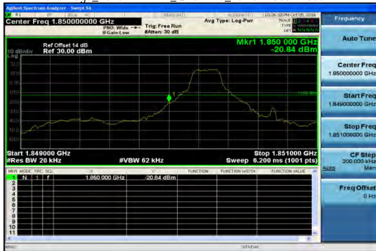
Band Edge_Band2 1.4MHz_QPSK 1 0_LowCH18607-1850.7
