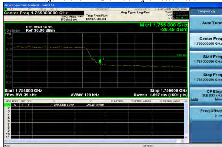
Band Edge_Band4 3MHz_QPSK 15 0_HighCH20385-1753.5
