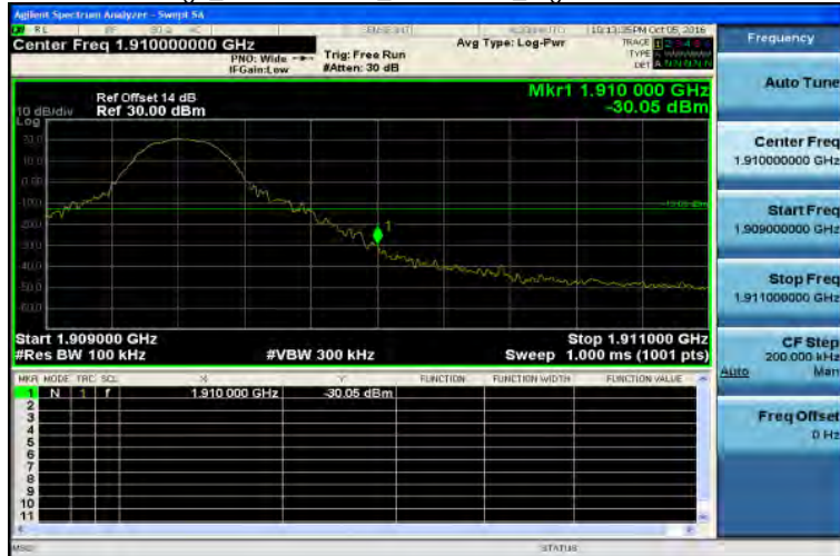
Band Edge_Band2 10MHz_QPSK 1 49_HighCH19150-1905
