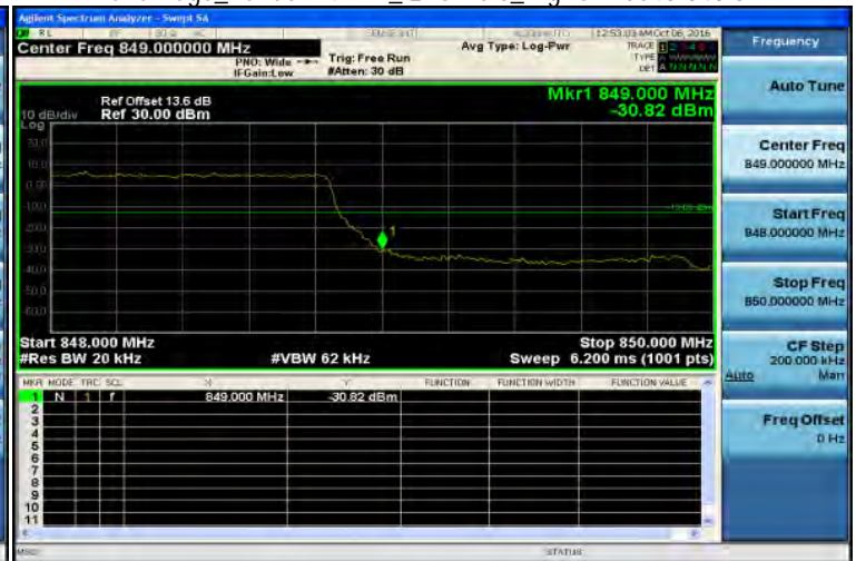
Band Edge_Band5 1.4MHz_QPSK 6 0_HighCH20643-848.3
