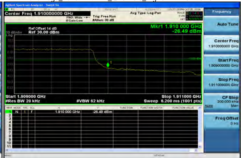
Band Edge_Band2 1.4MHz_QPSK 6 0_HighCH19193-1909.3
