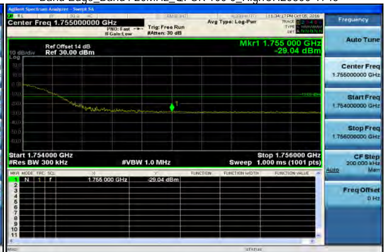
Band Edge_Band4 20MHz_QPSK 100 0_HighCH20300-1745
