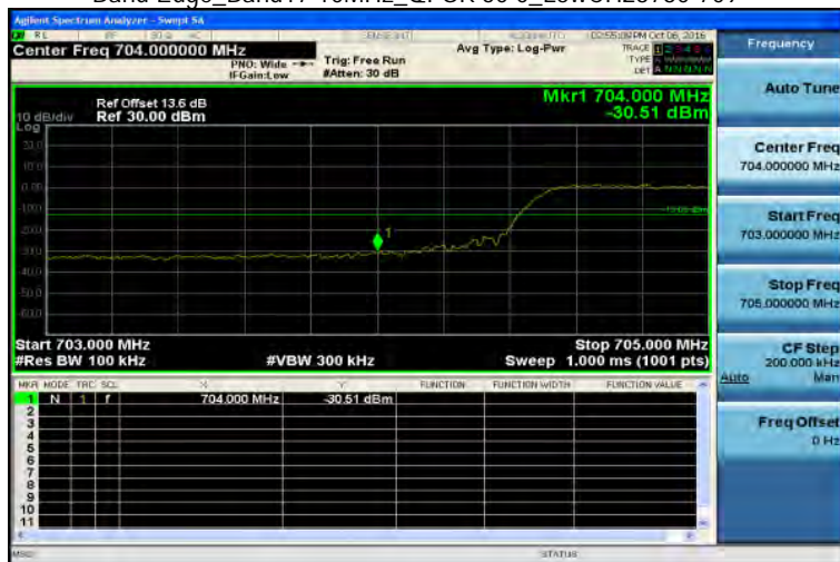
Band Edge_Band17 10MHz_QPSK 50 0_LowCH23780-709
