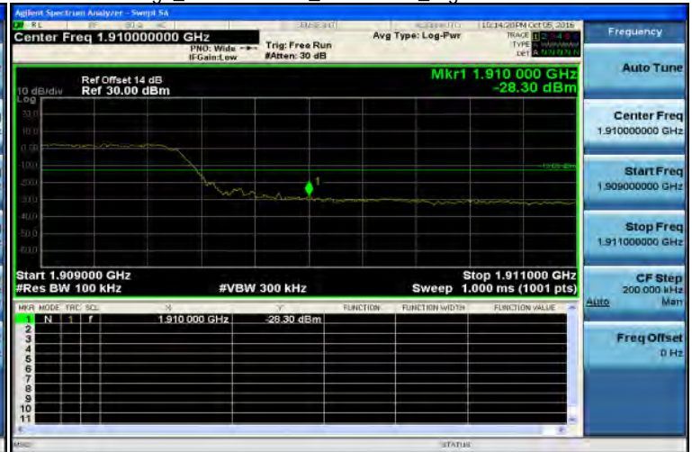
Band Edge_Band2 10MHz_QPSK 50 0_HighCH19150-1905
