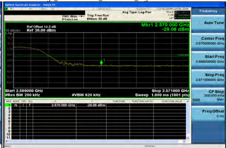
Band Edge_Band7 15MHz_QPSK 75 0_HighCH21375-2562.5
