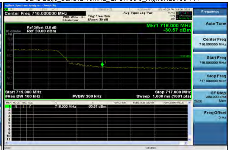
Band Edge_Band12 10MHz_QPSK 50 0_HighCH23130-711
