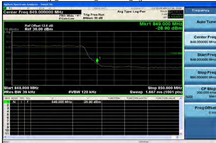
Band Edge_Band5 3MHz_QPSK 15 0_HighCH20635-847.5
