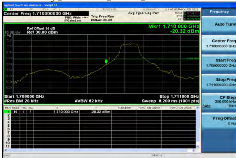
Band Edge_Band4 1.4MHz_QPSK 1 0_LowCH19957-1710.7
