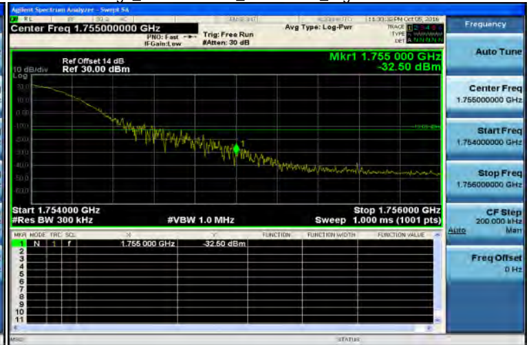
Band Edge_Band4 20MHz_QPSK 1 99_HighCH20300-1745
