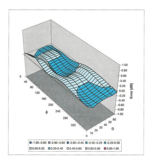
Spherical Isotropy Error < ± 0.4 dB
