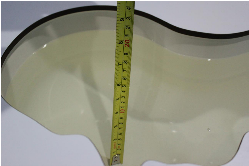
Picture 8.7 Liquid depth in the Head Phantom (5GHz)
