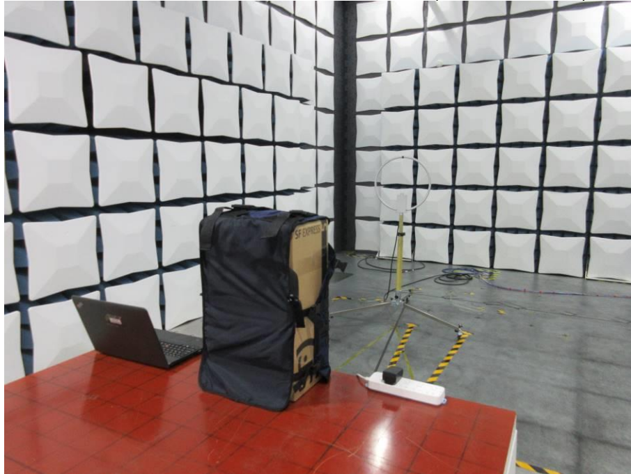
RADIATED RF MEASUREMENT SETUP (9KHz ~ 30 MHz)
