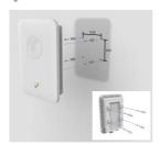
Drill 4 holes of Ø6mm (Ø0.25"Inch) on wall. Press fit plastic anchor and assembly fastener. Leave 5mm to 6mm gap between wall and fastener head. Use the four mounting slots given on the back of the radio to mount to the wall.
