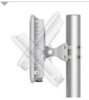
Align Radio to required angle by tilting up and down. The maximum radio tilting angle is  $\pm$  40°, with an incremental of 10°.
