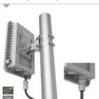
Insert RJ45 to radio housing and the lock cable gland to radio housing with 1.5Nm to 2Nm torque.
