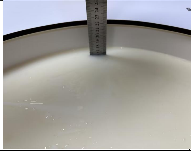
Photo 1: Tissue Simulant Liquid for Head 700-3000MHz
