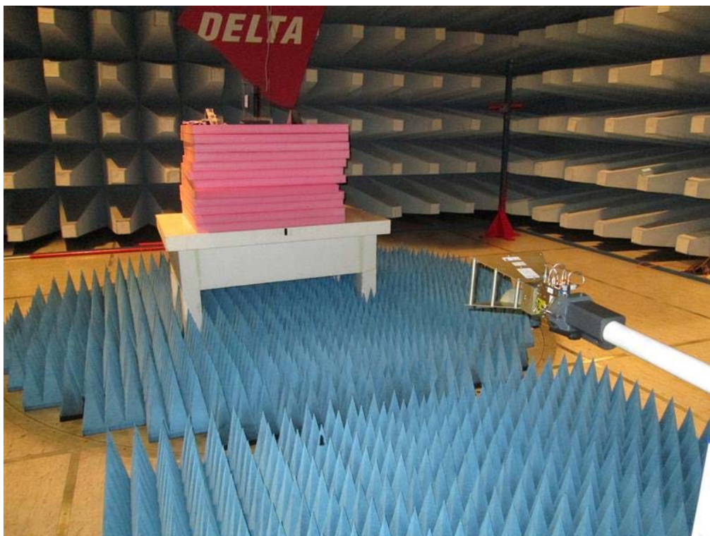
Photo 4.2.1 Test setup regarding measurement of radiated emission above 1 GHz.
