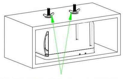
4: Install gasket and tighten nut
