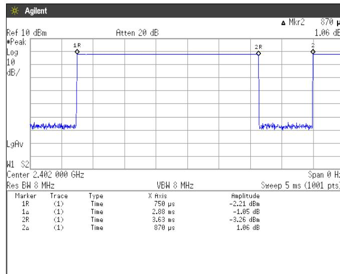
$$\text{Duty Cycle} = \text{Ton} / (\text{Ton} + \text{Toff}) = 2880[\mu\text{s}] / (2880[\mu\text{s}] + 870[\mu\text{s}]) = 76.8[\%]$$
