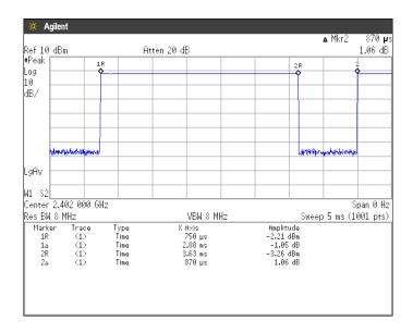
Duty Cycle = Ton / (Ton + Toff) =  $2880[\mu s] / (2880[\mu s] + 870[\mu s]) = 76.8[\%]$
