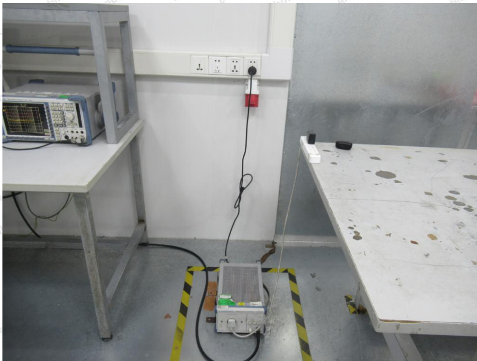
Photo of Conducted Emission Measurement
