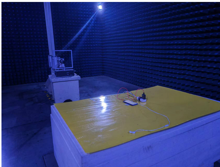
Photo of Radiated Emission Measurement (30MHz-1GHz)
