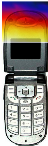
Figure 28 Sample H-field Scan Overlay
