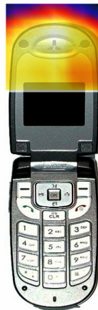
Figure 27 Sample E-field Scan Overlay
