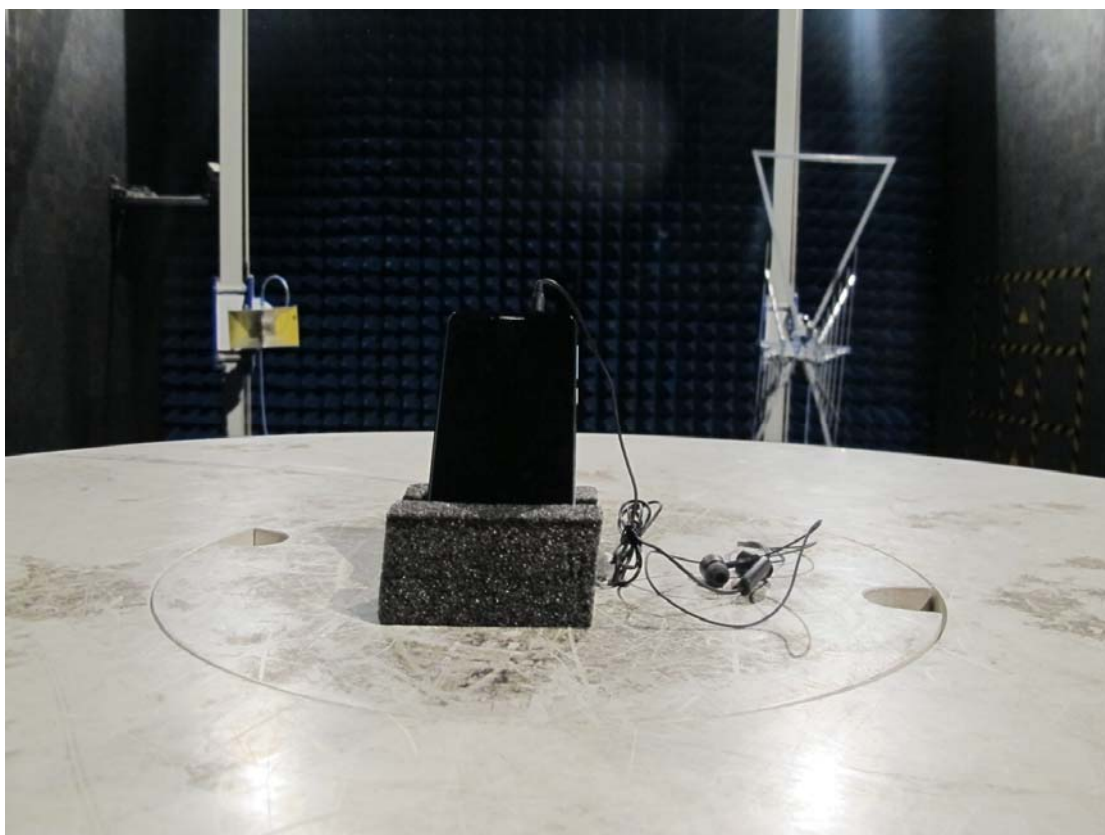
Radiated Spurious Emissions Test setup
