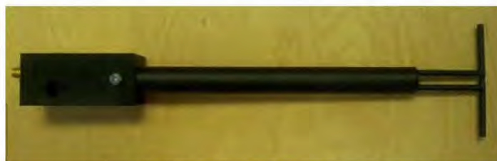
Figure 1 – MVG COMOSAR Validation Dipole
