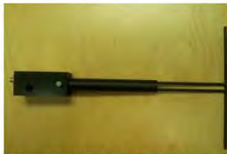
Figure 1 – MVG COMOSAR Validation Dipole
