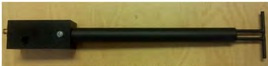
Figure 1 – MVG COMOSAR Validation Dipole
