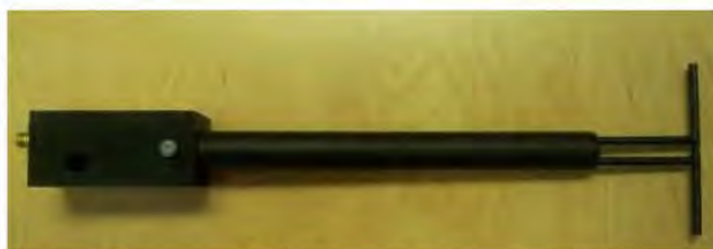
Figure 1 – MVG COMOSAR Validation Dipole
