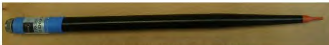
Figure 1 – MVG COMOSAR Dosimetric E field Dipole
