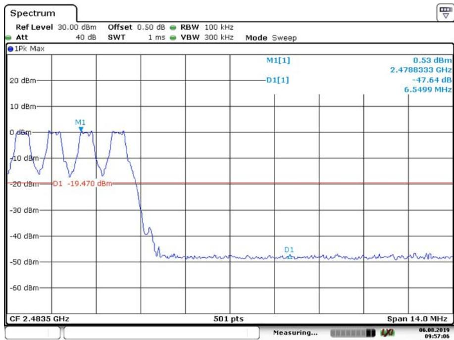
2EDR Mode ( $\pi/4$ -DQPSK):**Band Edge, Left Side**
