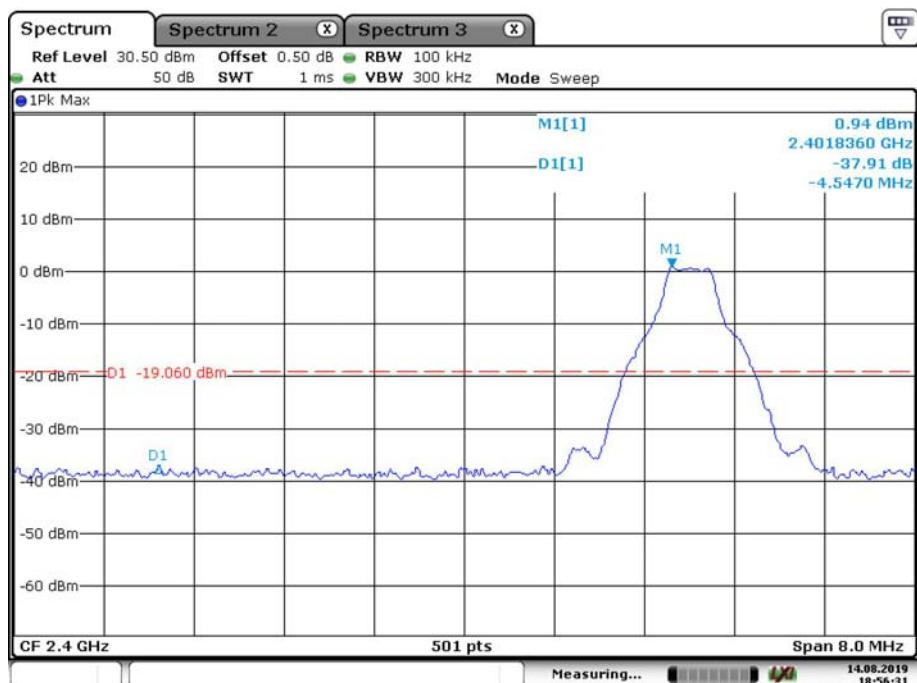
**Band Edge, Right Side**
