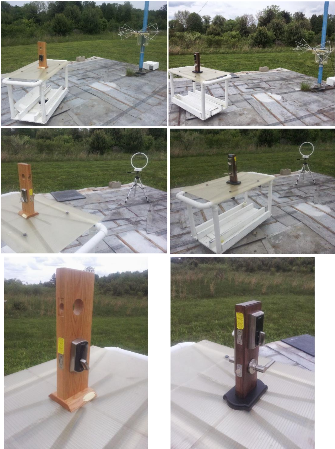
Figure 4: Radiated Emissions Test Setup Photograph(s).
