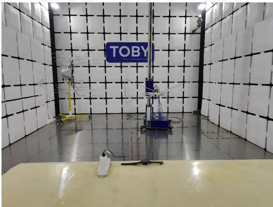
Photo of Setup for Radiated Emission (30MHz~1GHz)
