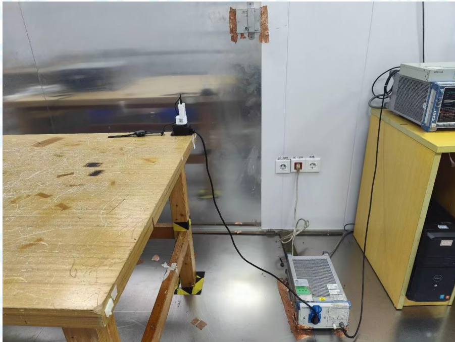
Photo of Setup for Radiated Emission (30MHz~1GHz)
